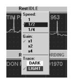
Defaults will be set at the factory of a speed equivalent to 25mm/sec and a gain of 1mv. Options for speed are  $\frac{1}{2}$  - equivalent to 25 mm/sec, 1 – equivalent to 50 mm/sec, and  $\frac{1}{4}$  - equivalent to 12.5 mm/sec. Options for Gain are x1 – 1mv, x2 = 2mv, and x4 = 4mv. The waveforms cannot be made smaller than 1mv.
