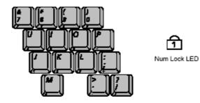
Press **press** to turn on the embedded numeric keypad. The numeric functions of the keypad are enabled and the Num Lock LED turns on. (See "Reading the System Status Lights" on page 20 for the location of the Num Lock LED.)
