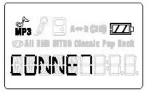
'CONNECT' will be displayed on the LCD display if it is connected normally.
