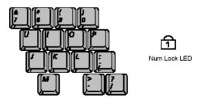
Press to turn on the embedded numeric keypad. The numeric functions of the keypad are enabled and the Num Lock LED turns on. (See "Reading the System Status Lights" on page 20 for the location of the Num Lock LED.)
