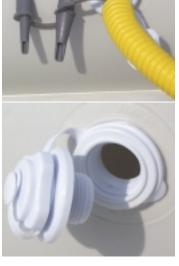
To deflate, unscrew the inner valve and remove. Most of the air will rush out in a minute or two, and any remaining air will be forced out when the boat is rolled up for storage.
