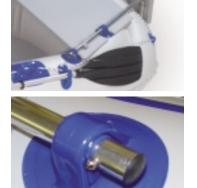
For the Sea Eagle 6, insert a clevis pin through the holes on the long top tubes to lock in place with retainer rings. The bottom rods are secured as follows: from the inside of the tube, push clevis pins through the holes and thread the retainer rings through them.
