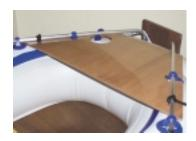
The Motormount Support Bench is a comfortable seat that improves support for heavier outboard motors. It also transmits the rotational force of the engine and reduces tran-
