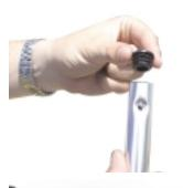
Insert the longer end of each rod through the two motor-mount grommets on the top stern section. Insert the shorter ends through the bottom grommets.
