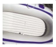
1. Inflate both chambers in the inflatable floor fully. If the inflatable floor is not fully inflated the floorboards will have a small gap on either side. Inflate chambers 1 & 3 to 60-75% of maximum pressure. You should be able to push 4 to 5 inches into the hull.
