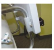
Holding the wood motormount block to the back of the rods, place the U shaped clamps on the inside of the tubes. Insert a bolt through the clamp on each side and fasten with a knurled nut & washer behind the board. Make sure the motormount block is mounted at the highest position.
