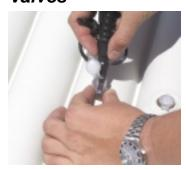
**Pipe Valve:** Sea Eagle pipe valves are simple, reliable and compact. Insert the cone shaped nozzle on your pump to inflate.
