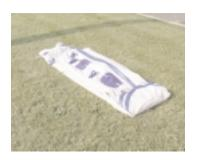
Starting from the bow, roll toward the stern of the boat tightly to force out any remaining air.
