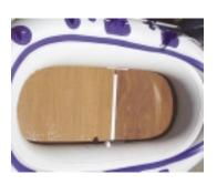
5. If you are not installing a motormount, reinflate your boat by first pumping up chamber 1 and then chambers 2 & 3. Your floorboards should fit tightly to the hull of your boat and provide excellent stability.
