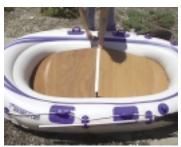
2. Place floorboards inside the boat. The boards will overlap when laid flat over the floor. Lift both boards and place them in the aluminum H-bar connector. The boards should be in an inverted V.
