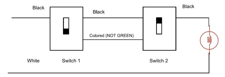
Wrong Z-Wave switch position for typical 3-way
