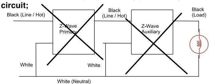
Correct Z-Wave switch position for typical 3-way
