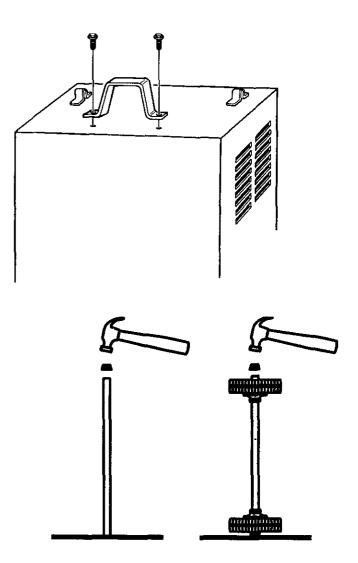
2. Hold axle upright on floor or work surface. Then, using a hammer, tap one of the plastic hubs onto the top end of the axle. Be sure to tap the hub on straight. Slide both wheels onto the axle with the hubs facing inward.
