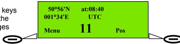
In 'normal' mode ('standby screen'), the **Left Action key** and **Right Action key** have the functions **Menu** and **Pos**, respectively.
