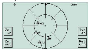
This screen shows all received AIS stations and their velocity vector. The top left number is the number of stations within the range of the display. The range, shown at top right, corresponds with the outer ring of the displayed graphic.
