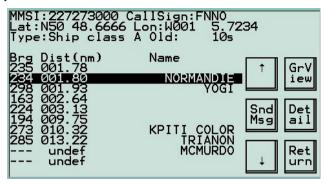
Individual targets can be viewed in more detail in 2 ways. Highlight a target; at the top of the screen more detailed information can be seen about the selected target. For full details, highlight the target and press **Detail**
