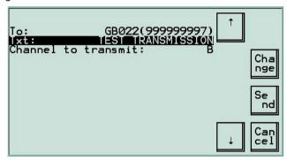
To test the system, select a coast station and compose a message, for example: "This is an AIS test call, please acknowledge".
