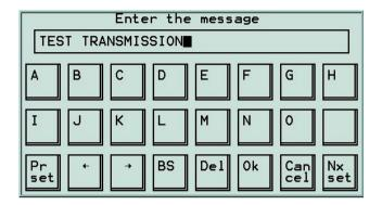
When the message has been entered correctly, select **OK**. Select **Send** to transmit the message.
