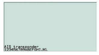
After successful completion of the self-test and communication between the VDU and the transponder has been established the following screen will appear.
