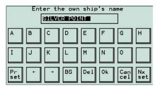
To confirm the change in ship's name the system password must be entered. (See section 4.8 Setup System Password on page 36)
