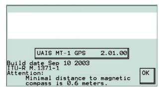
The welcome screen giving the GNSS type (GPS or GLONASS), software version, and software build date then appears, which confirms that the VDU is ready for operation.
