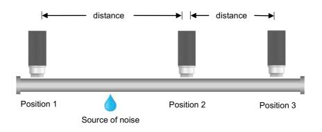
There must be one sensor "in front of" the sound source (Position 1). There must be two sensors "behind" the sound source (Positions 2 and 3).
