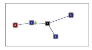
The correlation of the line from sensor 5 to 3 results in a leak at the very same position.
