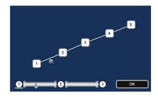
**Example 2:** The source of noise is located between the sensors 2 and 3. Possible entry on the Correlator: first, sensor 2, then sensors 3 and 4.
