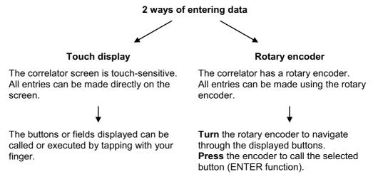
You can always switch between operating via touch screen and operating via rotary encoder.
