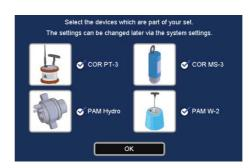
The statements made here determine which measuring methods will be offered in the Correlators Start screen.
