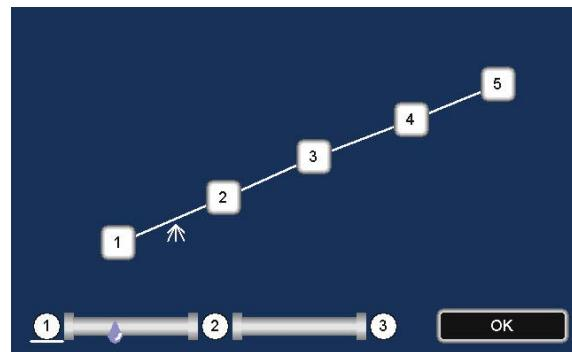
**Example 2:** The source of noise is located between the sensors 2 and 3.
