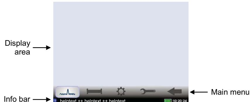
**Main menu** Using the buttons in the main menu bar you can access the individual functions of the device.
