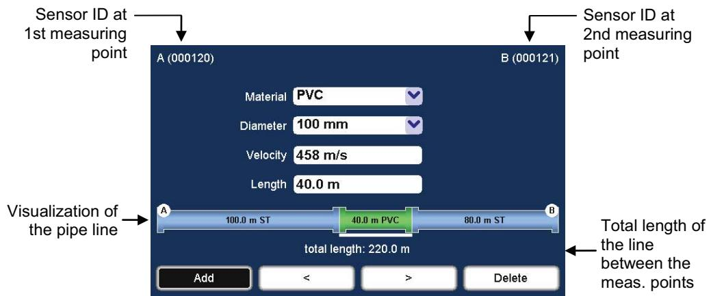
**Drop-Down Lists:** Material ... Select the pipe section's material.
