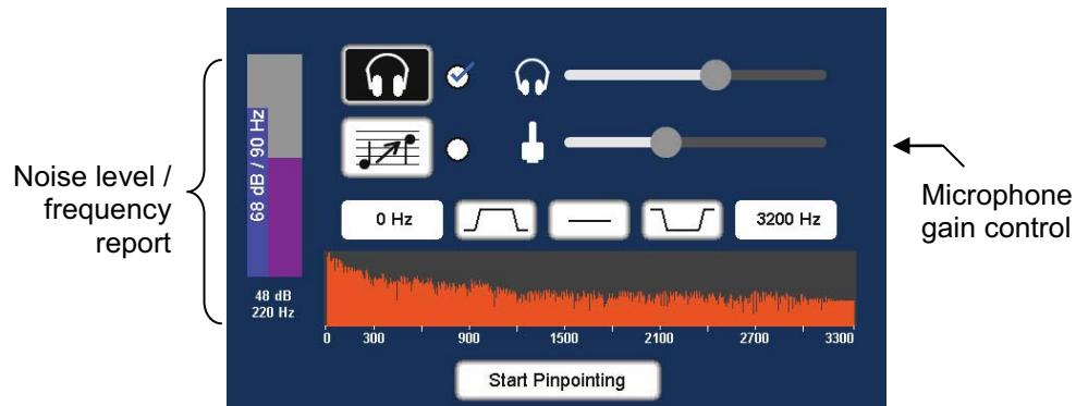
On the left, the **Instantaneous value** and the **Minimum value** of the current measurement are displayed.
