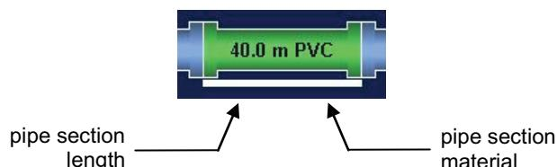
The selected pipe section is "highlighted" with a white bar. The pipe parameters in the four input fields refer to this section.
