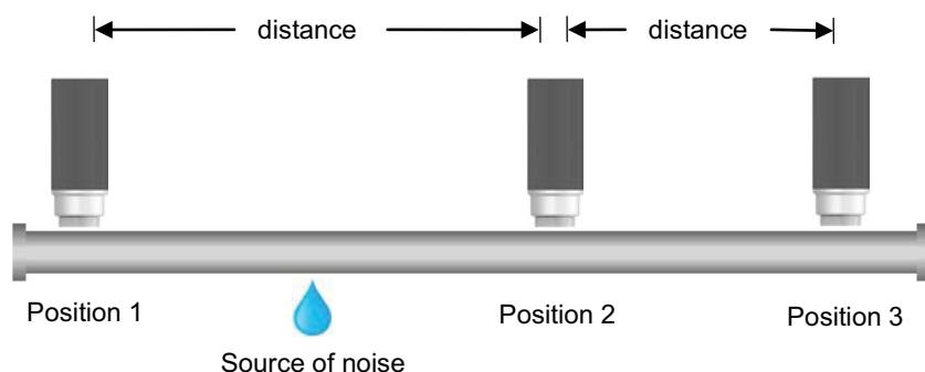
There must be one sensor „in front of“ the sound source (Position 1).
