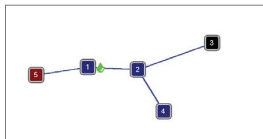
The correlation of the line from sensor 5 to 1 shows the drop icon right at sensor 1.
