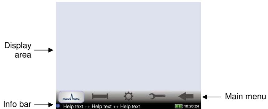
*Main menu* Using the buttons in the main menu you can access the individual functions of the device.
