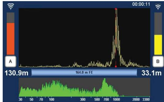
In the Correlation menu, Power transmitter A appears on the left, Transmitter B appears on the right.
