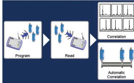
**Result:** A "Multi correlation" is carried out, which means that the values of all sensors are correlated with each other. The process can take a few seconds. Subsequently, the correlation results for all sensor pairs are shown in thumbnails.
