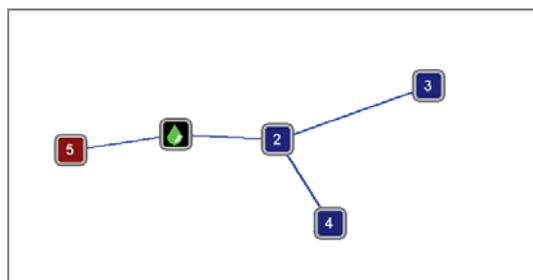
The correlation of the line from sensor 3 to 4 shows the drop icon right at sensor 2.
