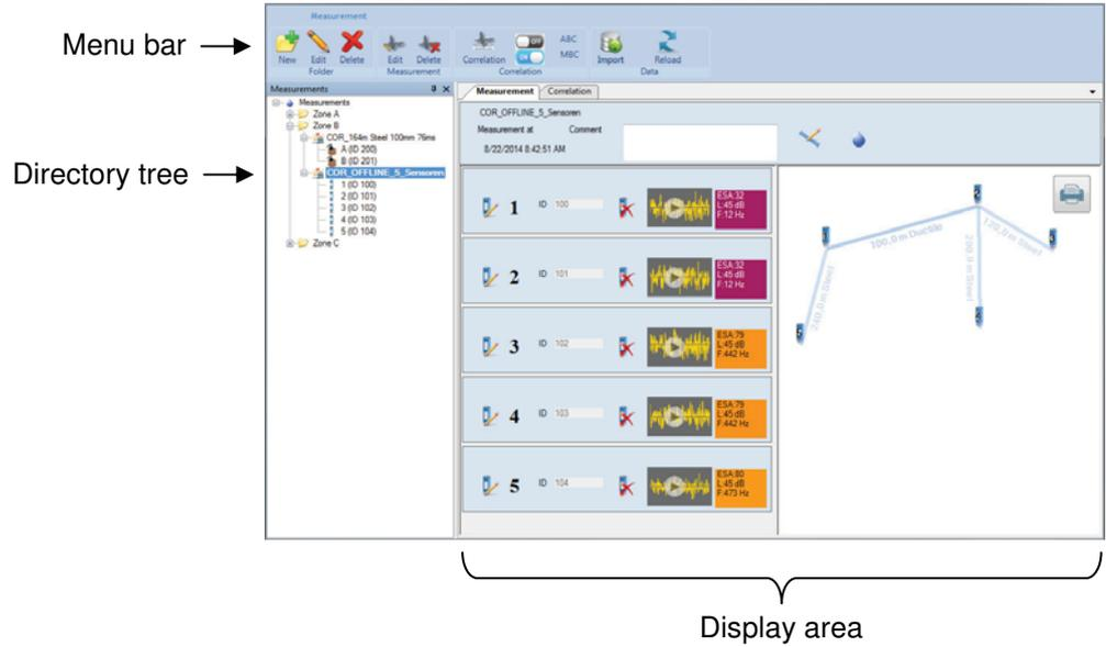
**Menu bar** The menu bar (ribbon) allows you to access any command or function. Function keys are combined appropriately into different segments. The CorreluxView symbol at the top left of the menu bar allows you to access system settings for the application.
