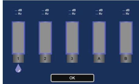
As long as the pinpoint location is in progress, in regular periods the currently measured value of each sensor is retrieved by the Correlator and displayed. In addition, the lowest measured value (Minimum value) of the current measurement is displayed for each sensor.
