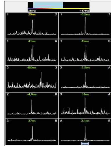
*Set frequency filters* The frequency diagram at the very top of the screen allows you to set a frequency filter and to repeat the correlation.
