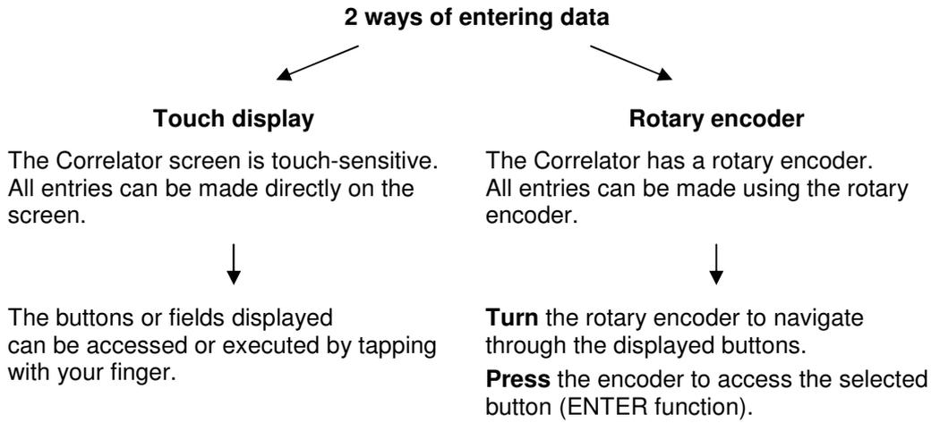
You can always switch between operating via touch screen and operating via rotary encoder.
