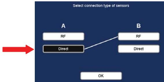
Variant 2: The measurement shall be performed without Power transmitter B? Then tap the **Direct** button beneath **B** and confirm with **OK**.
