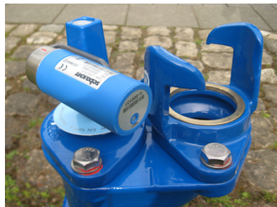
Logger with an angle adapter horizontally on the valve rod
