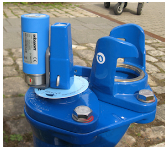
Logger with an angle adapter on the valve rod
