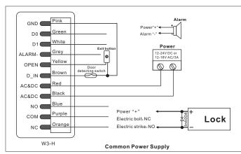
Connect the negative pole of the lock to NC is for Fail safe lock. Connect the negative pole of the lock to NO is for Fail-secure lock.
