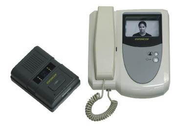
Easily connect an additional monitor and/or an additional camera Secondary Monitor: **DP-121-SQ** Additional Camera: **DP-121-CQ**  SECO-LARM's Video Door Phone displays an image of the visitor in real time on the phone's monitor, and a built-in microphone and speaker on the camera unit lets users communicate with visitors. Authorized visitors can then be granted entry with the push of a single button.
