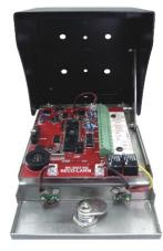
Unique faceplate hinge allows for easy installation.
