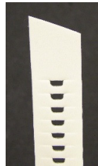
Figure 1.2 Strap cut at 45° angle
