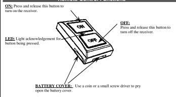
BATTERY REPLACEMENT: Open the battery cover with a coin or screw driver. CR2032 can be replaced once low.
