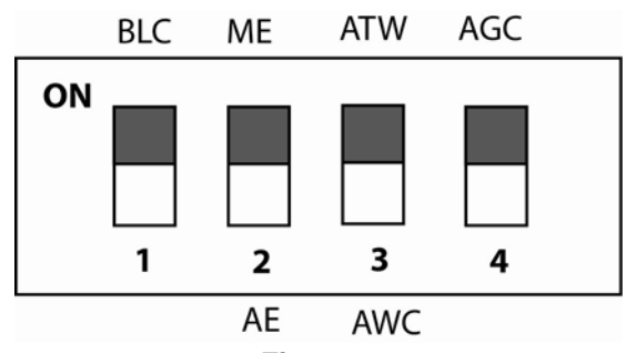
Figure 8 Default DIP Switch Settings for the Color and Day/Night Cameras Only
