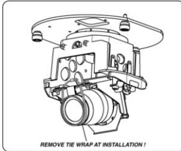
Figure 3A Tie Wrap Location
