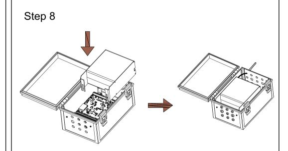
Put the battery holder into the sensor box. Screw the butterfly nuts. Plug the battery cable to the battery header on mainboard.
