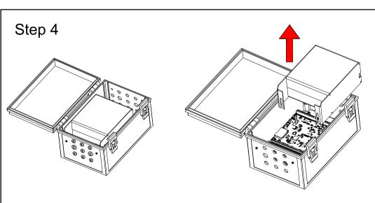
Open the sensor box, unplug the battery cable from the mainboard, unscrew two butterfly nuts on the side of battey box, then take out the battery holder box.
