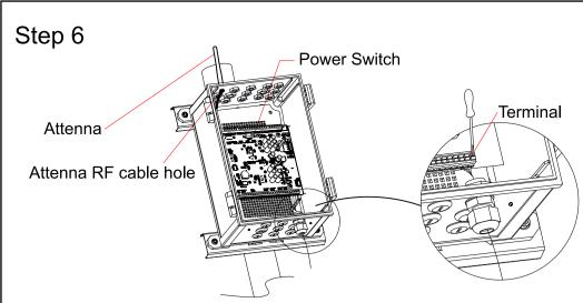
Insert the cable gland with wire into the hole. Connect the wire to the mainboard terminal based on the wire color, use a screwdriver to fix the wire.
