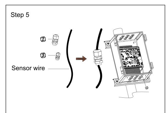
Disassemble one of the hole plugs on the sensor box. Select one PG9 or PG7 cable gland according to the hole size, insert the sensor wire into the gland hole.
