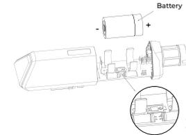
**Note:** Do not invert the positive and negative batteries. Otherwise, short circuit may occur and the device may be damaged.
