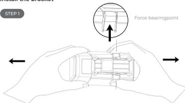
One hand holds the clasp while the other holds the device. Pull outward with opposite force.
