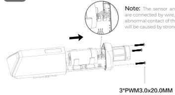
**Note:** The sensor and PCBA are connected by wire, and the abnormal contact of the sensor will be caused by strong pull.
