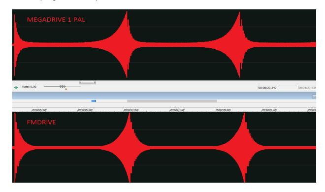
Technical manuals claim that AR should be 31 (no attack) when using SSG...however setting an attack phase and producing this behavior can be used in a creative way.
