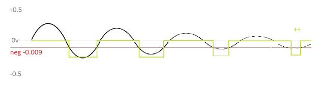
What I have found during close experimentation on the real chip is that the distorted part is actually here even when the output register for a channel are zeroed out. This leads me to search for an analog problem then trying to do basic reverse engineering; I have implemented a "negative value bug" that reproduces the effect closely, especially at the very end of an envelope where the signal period also change...
