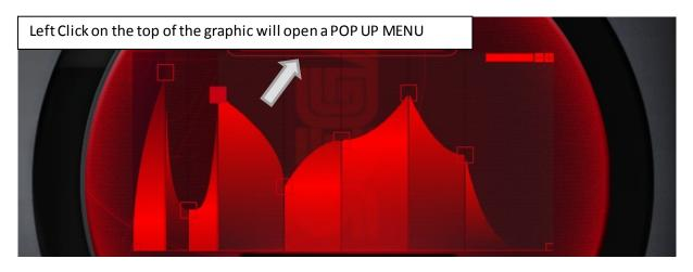
Extended feature of FMDRIVE allows the use of custom complex envelopes instead of the original parametric. (can be done on a real YM2612 by sending software envelope data to TL register)
