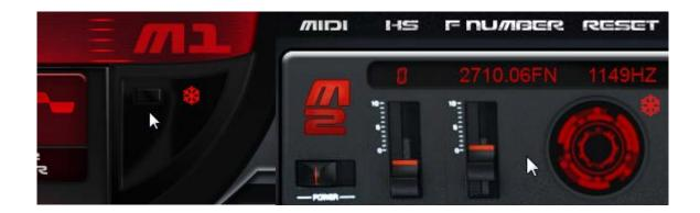
Activating the MIDI switch next to an OPERATOR allows frequency and key on / off happening independently. Controls are made by a different MIDI channel for M2, C1 and M1.
