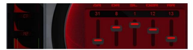
The sound starts when the key is depressed, a process called 'key on'. The sound has an attack, a strong primary decay, followed by a slow secondary decay. The sound continues this secondary decay until the key is released, a process called 'key off'. The sound then begins a rapid final decay, representing for example a piano note after the key has been released and the damper has come down on the strings.
