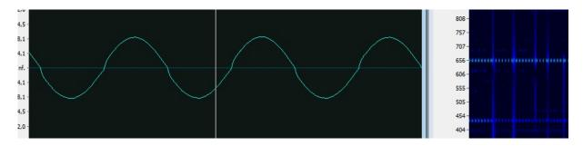
When using MD1 Model the **Overdrive parameter** allows to fine tune the effect to taste, *most notably when ALGO 7 is in use, the output might distort too much*. (Different Sega models and revision will produce different result in real world.)
