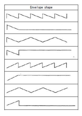
The phase is also reset in SSG mode at the beginning of each repetition of the waveform in cases where both the HLD and ALT bits are unset. This produces different harmonic results when the envelope is very short.
