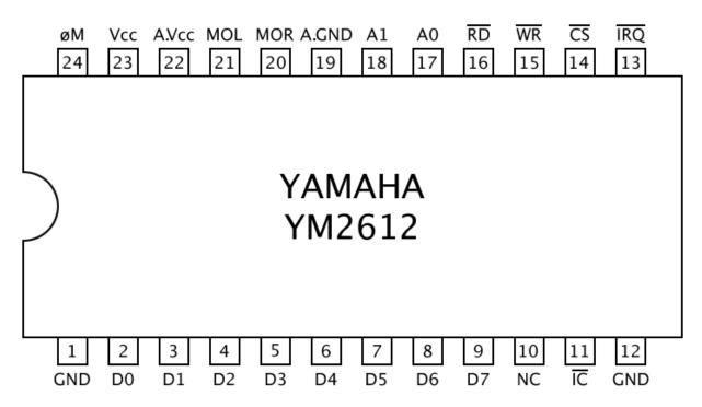
The **YM2612**, aka **OPN2**, is a six-channel sound chip developed by Yamaha. It belongs to Yamaha's OPN family of FM synthesis chips used in several game and computer systems.
