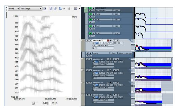
A practical way for using the CSM mode is MIDI automation. Use Midi Channels 11, 12, 13 and 14 in your DAW to control Operators frequencies and Timer A by Midi notes. Pitch bend values can add to the natural vocal tone of the sound.
