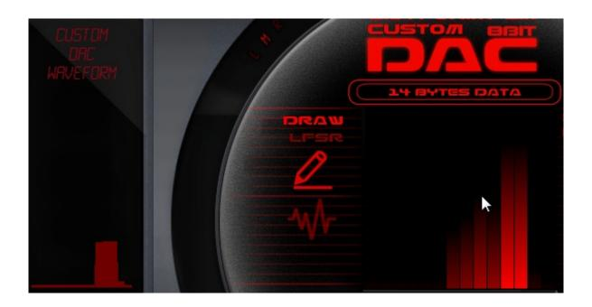
14 bytes of data can also be directly written to the DAC allowing the use of raw custom waveforms.
