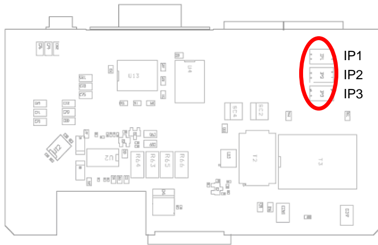
Back card deep switch positioning
