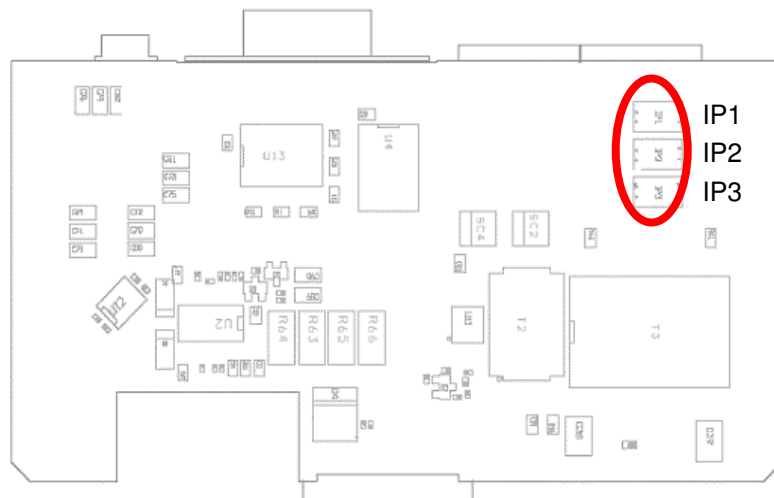
Back card deep switch positioning
