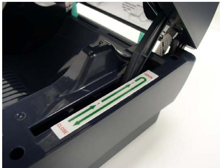
Fig. 1 Top cover support is fixed at position 2
