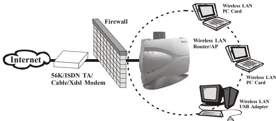
Figure 1-6 Wireless router and IP Sharing
