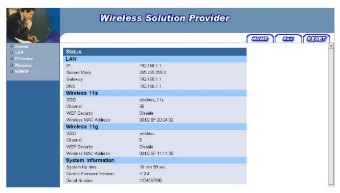
There are three tabs on the upper right-corner of each page. To go back to the main setting page, press HOME tab. To log out of the web management, press EXIT tab. To complete any change you have made, press RESET tab after clicking APPLY button.
