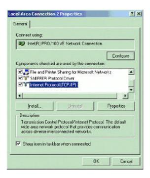
2. Make sure the IP address of your computer and the AP are in the same subnet. The default IP address of the access point is 192.168.1.1 and the default subnet mask is 255.255.255.0.
