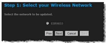
Specify the Wireless Network Name (SSID) for the device. The SSID is a unique named shared amongst all the points of the wireless network. The SSID must be identical on all points of the wireless network and cannot exceed 32 characters. Click on the Next button to continue.
