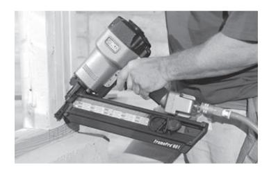
Sequential Actuation Trigger (also known as restrictive trigger or trigger fire) operates in the following a sequence - depress the safety element at the nose of tool against the work surface then pull the trigger. After each fastener is driven, release the trigger and lift the tool off the work surface before starting the sequence again. This trigger is recommended and acceptable for most applications.
