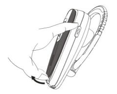
Slightly, open the cover from the gap of bottom of front housing
