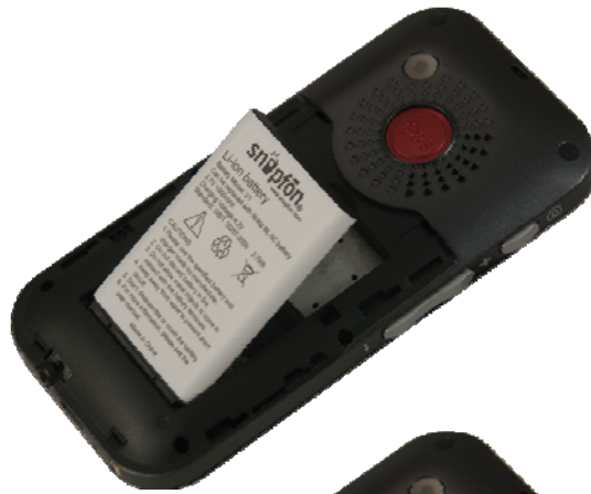
Figure 2. Battery Installation Diagram
