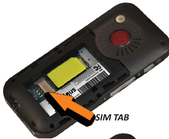
Figure 1. SIM Card Installation Diagram
