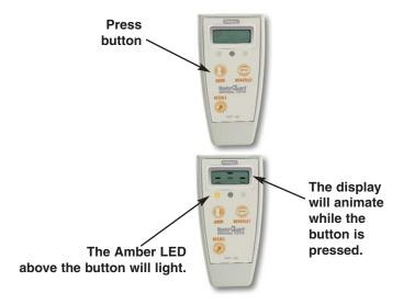
Repeat the button press or hold the button down for continous transmission.
