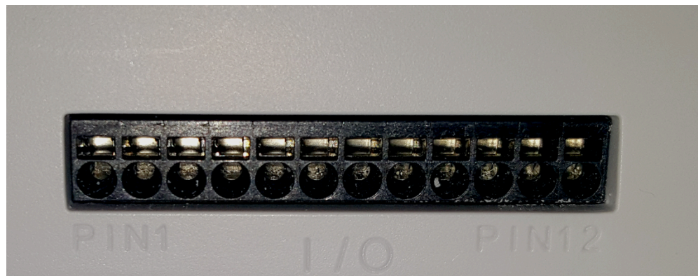
Figure 7 The GPIO port.
