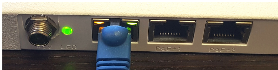
Figure 15 The SensArray+ has finished booting and is ready for operation. The LED is flashing green.
