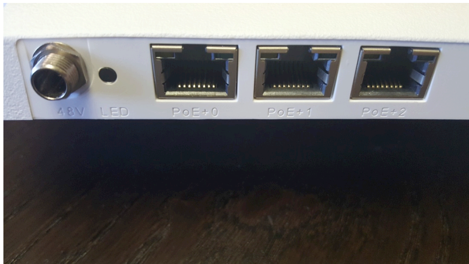
Figure 5 A closer look at the 48V input, the indicator LED and the Ethernet ports.
