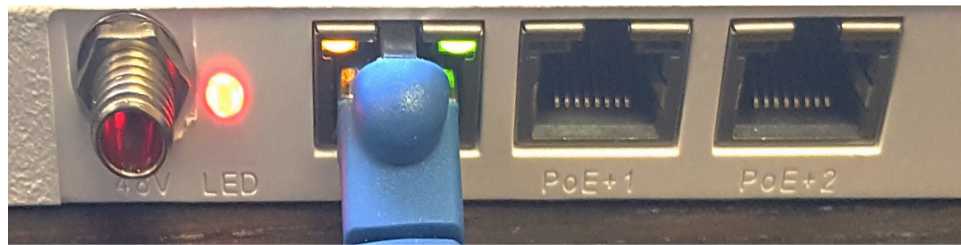
Figure 14 A SensArray+ in the process of booting. The LED flashes red.
