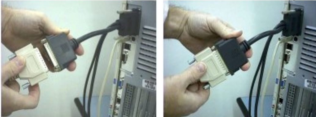
Figure 5a, b Reconnect Your Printer Cable, If Present
