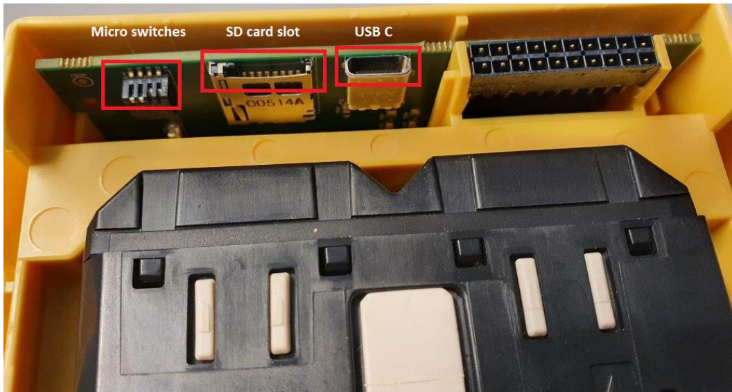
Figure 12 Swarm S2 datalogger: micro switches, SD card slot, and USB C port
