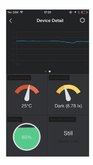
Step6: You can access to Yunzi's UUID, Major and Minor through this configuration tool and revise them according to your need. Through this app, you may also setup Yunzi's radius power, broadcasting frequency and even modify the operation parameters of the sensors.
