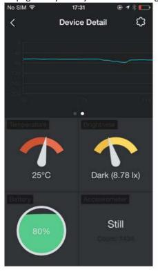
You can access to SmartBeacon's UUID, Major and Minor through this configuration tool and revise them according to your need. Through this app, you may also setup SmartBeacon's radius power, broadcasting frequency and even modify the operation parameters of the sensors.
