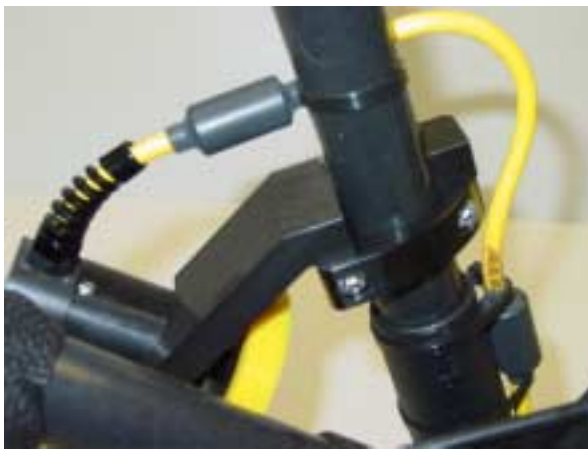
Figure: 4-6 If the odometer wheel does not make good contact with the wheel, use a hexagonal wrench to loosen the 2 screws (left) and pivot the odometer outward so when the wheel is attached the odometer rolls continuously (right).
