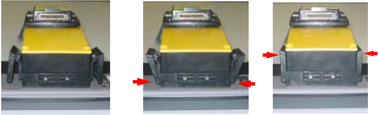
Figure: 3-3 Latching the electronics to the antenna.
