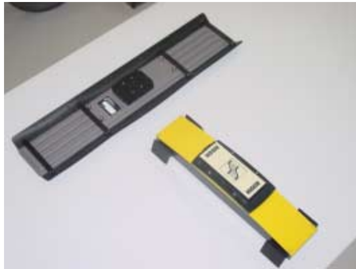
Figure: 3-1 Noggin 100 assembly of electronics to antenna.
