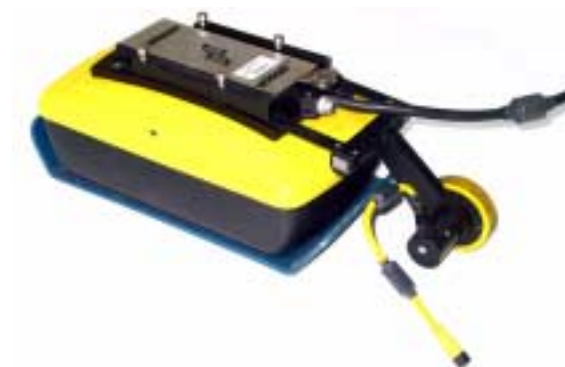
Figure: 6-3 Connect the 37 pin connector on the Noggin-to-DVL cable to the 37 socket receptacle on the Noggin unit by tightening the latch.
