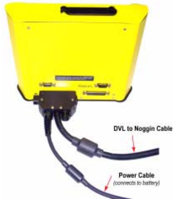
Figure: 9-3 The DVL-to-Noggin cable connects to the back of the DVL.
