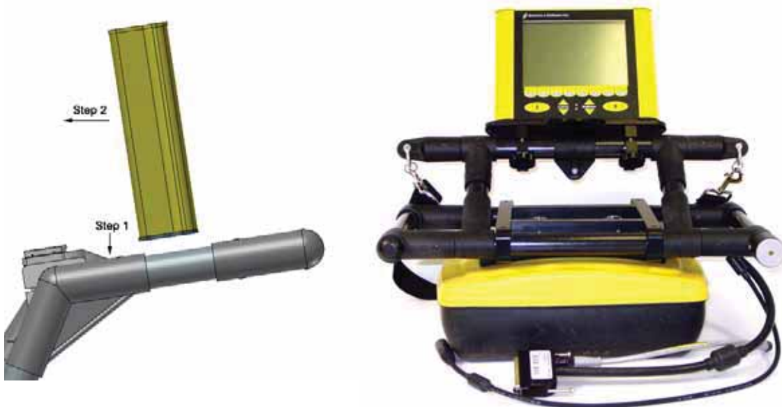
Figure: 8-11 Attach the Digital Video Logger to the frame. Attaching the digital video logger (DVL). Step 1: Depress flexible clip. Step 2: Slide DVL onto shelf.
