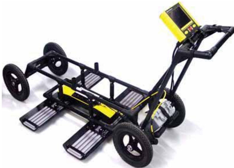
Figure: 5-11 After attaching the separation bars, place the SmartCart over the Noggin 100 system with the 8 antenna mounting posts inserted in the post blocks. The 37 socket receptacle on the Noggin 100 electronics must face the back of the SmartCart for the cable to connect properly.
