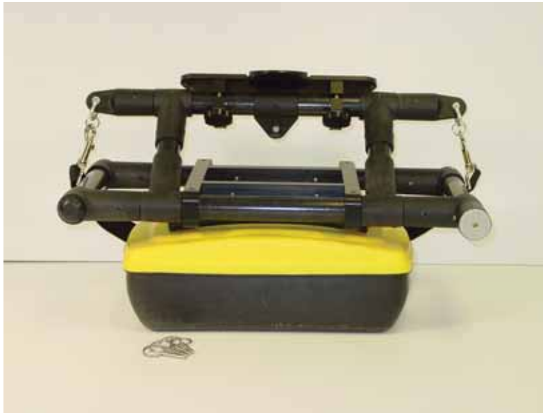
Figure: 8-8 Using the 4 holes on the bottom of the Rock Noggin frame, place the frame on the 4 mounting posts on the top of the Noggin (shown in Figure 8-6). Push the frame down until it cannot go any further. The Noggin should be oriented such that the 37 socket receptacle on the Noggin is on the same side as the SmartButton on the frame.
