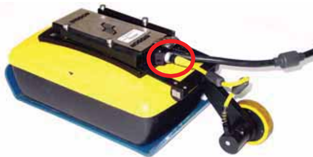
Figure: 7-4 On the Noggin-to-DVL cable, note the round receptacle on the back of the connector that attaches to the Noggin unit. Connect the yellow odometer cable to this round receptacle.
