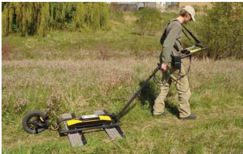
Figure: 6-2 Noggin 100 SmartTow configuration in use. Note the belt battery for power and DVL carrier for conveniently carrying the DVL in the field. The cable runs from the electronics housing and up the handle secured by velcro straps.
