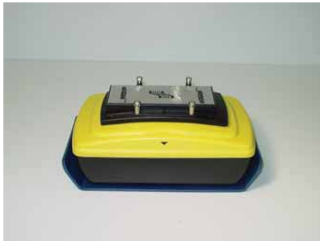
Figure: 15-1 Noggin with optional curved skid pad.
