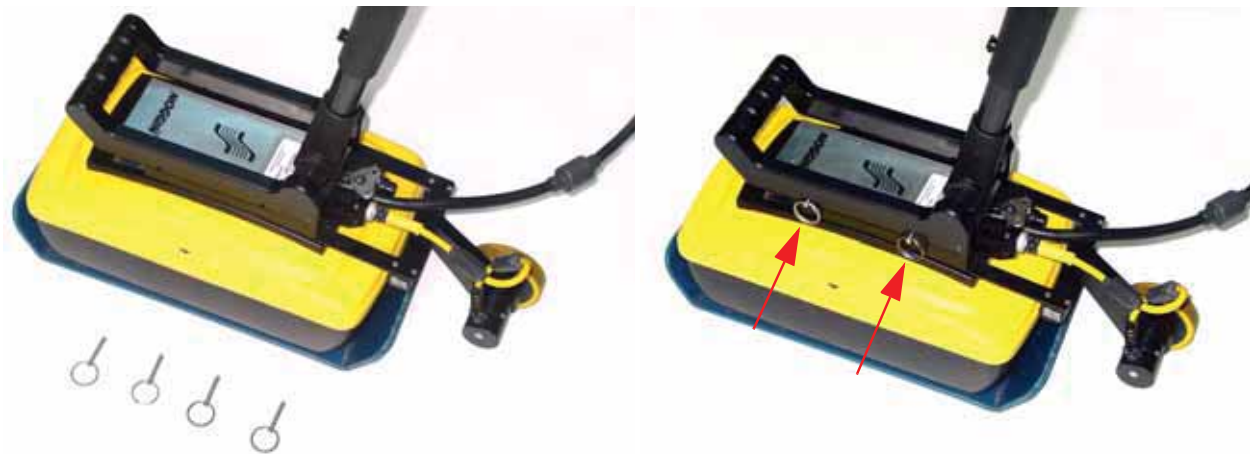
Figure: 7-5 Press the handle base straight down onto the four, silver mounting posts. The handle base should be pushed all the way down onto the odometer bracket. Insert the four quick-release pins to secure the handle.
