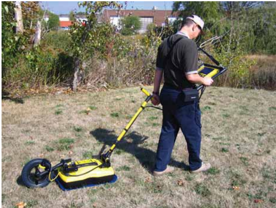
Figure: 6-9 Noggin 250 SmartTow in operation. Note the belt battery used to power the system.
