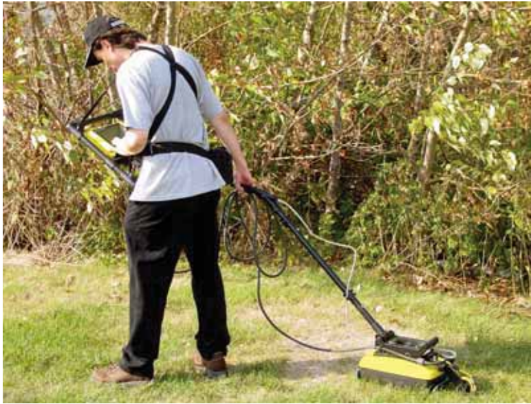
Figure: 7-7 In conditions where pushing the SmartHandle is difficult, it is possible to turn the handle around and pull the system as shown.
