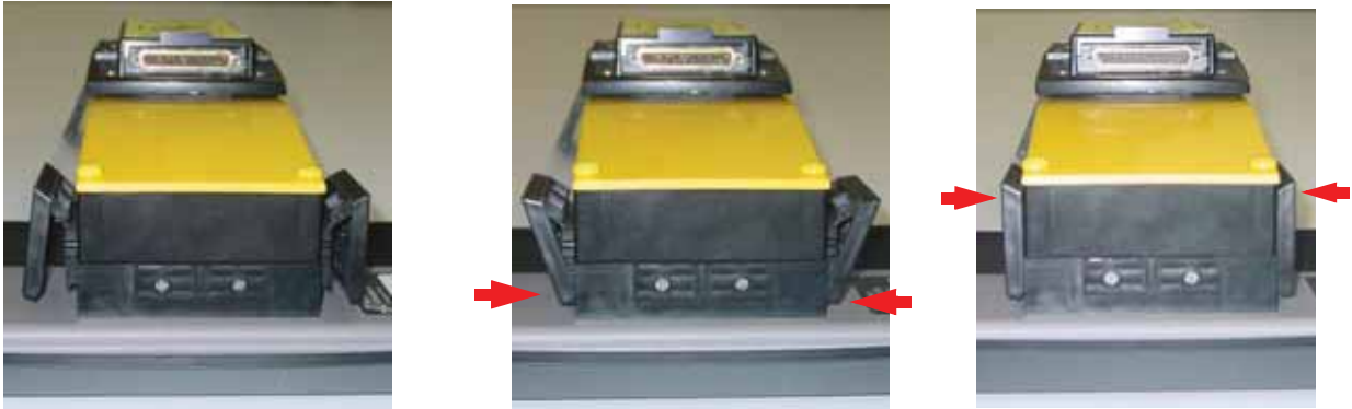
Figure: 3-3 Latching the electronics to the antenna.
