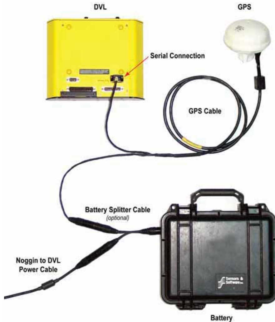
Figure: 9-1 GPS connect to the back of the DVL using a serial connection. GPS supplied with the system usually come with the optional battery splitter cable to power the GPS from the battery.
