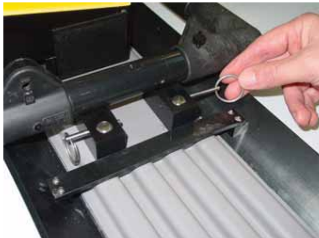
Figure: 5-12 Secure the SmartCart Separation Bars to the Noggin 100 by inserting the pins into each of the 8 post blocks.
