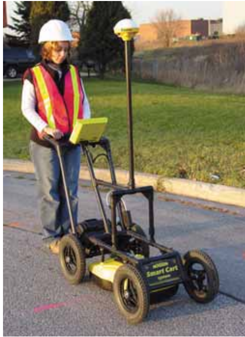
Figure: 5-16 SmartCart system with the optional GPS mounting bracket.
