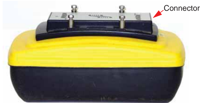
Figure: 8-6 The Noggin used with the Rock Noggin can be either a Noggin 500 (shown here) or a Noggin 1000. The connections are identical for both systems. The 4 silver mounting posts visible here are used when attaching the frame to the Noggin (see Figure 8-8).
