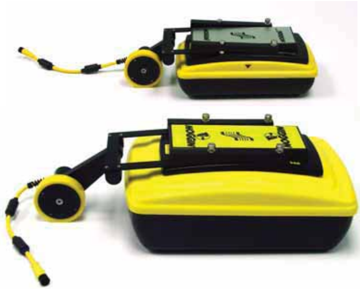
Figure: 7-2 Slide the Noggin odometer bracket over the four, silver mounting posts for both the Noggin 1000 (top) and Noggin 500 (bottom).
