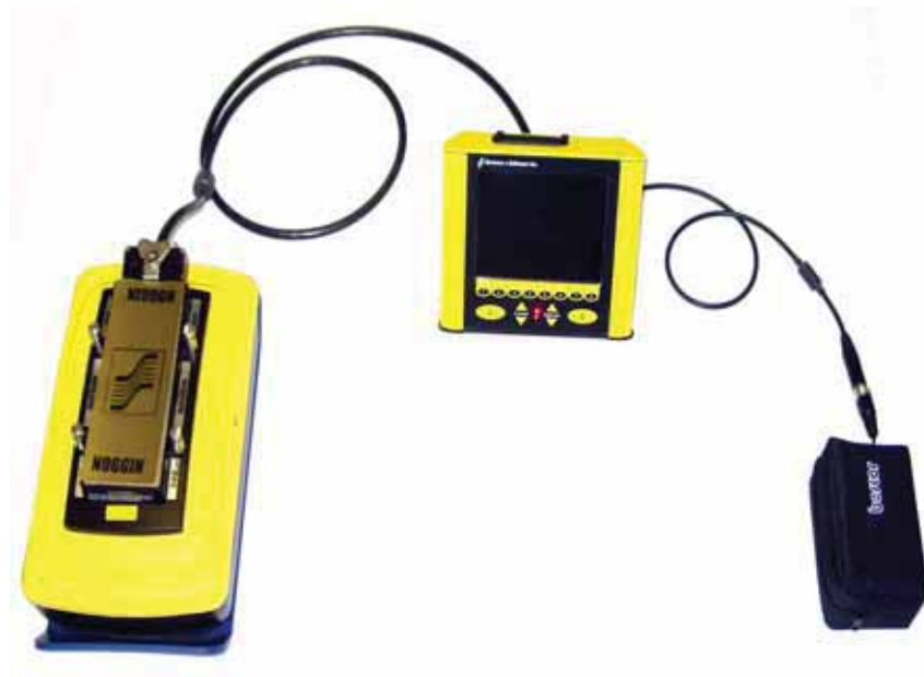
Figure: 4-2 Base Noggin system assembled.
