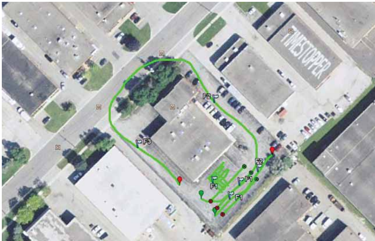
Figure: 13-14 Google Earth (KMZ) files display where the GPR data lines were collected as well as Fiducial markers.
