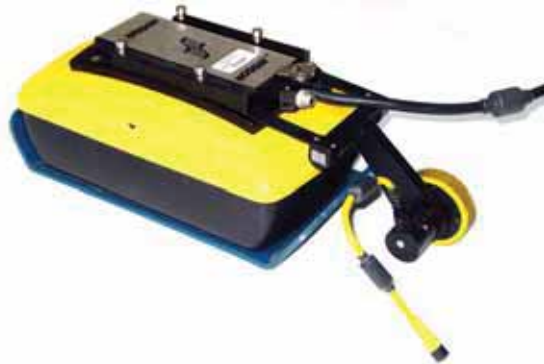
Figure: 7-3 Connect the 37 pin connector on the Noggin-to-DVL cable to the 37 socket receptacle on the Noggin unit by tightening the latch.
