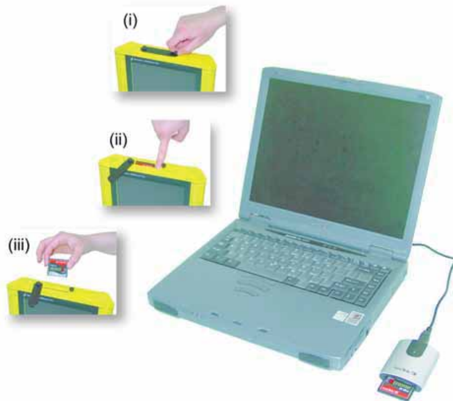
Figure: 12-2 Locate & Mark data images saved to the removable drive are easily transferred to a PC. First, power down the DVL, then (i) loosen both of the finger-screws on the top of the DVL so the drive door can swing open freely. (ii) Press the button to partially eject the compact flash drive. (iii) Remove the drive and insert it into a PC card reader (user supplied). Copy the image data folders from the drive into a folder on the PC using the Windows Explorer program. The optional GPR Image View program can then be used to view the data images.
