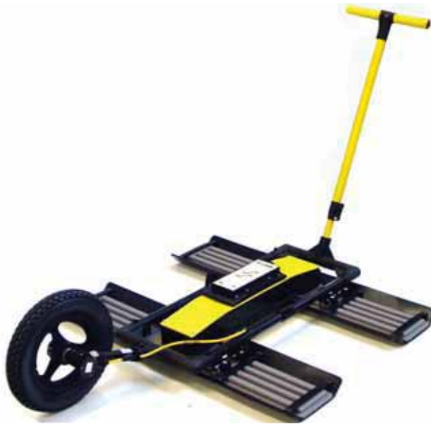
Figure: 6-1 Noggin 100 SmartTow configuration.
