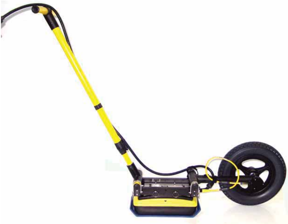
Figure: 6-10 Noggin 1000 in the SmartTow configuration
