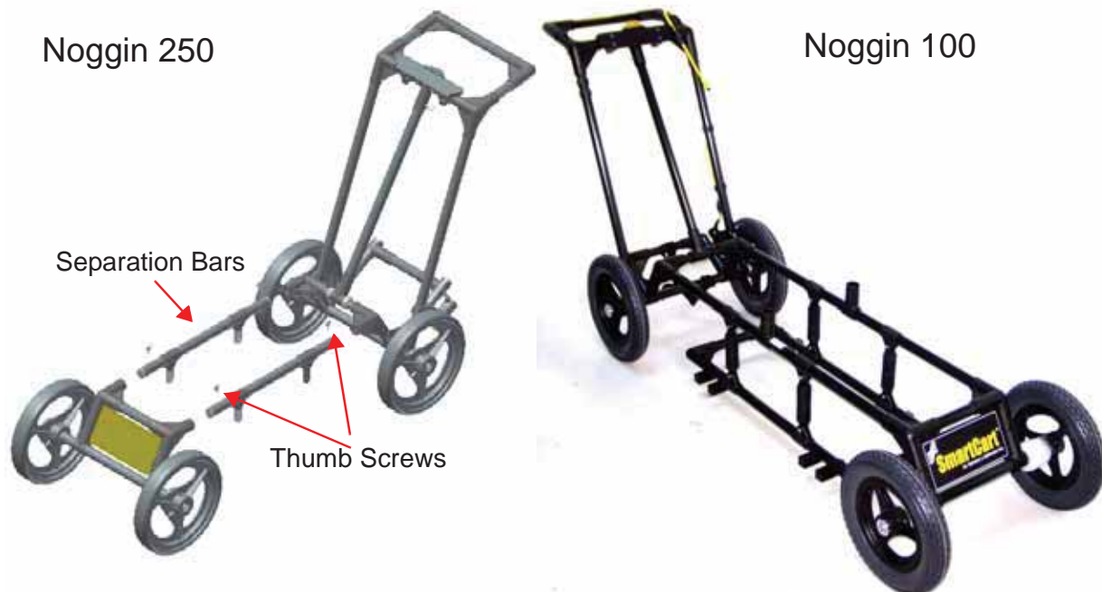
Figure: 5-7 The separation bars are attached to the SmartCart to carry the Noggin. Each Noggin system (100, 250, 500 and 1000) has a unique set of separation bars; the Noggin 250 separation bars are shown on the left and Noggin 100 separation bars on the right.
