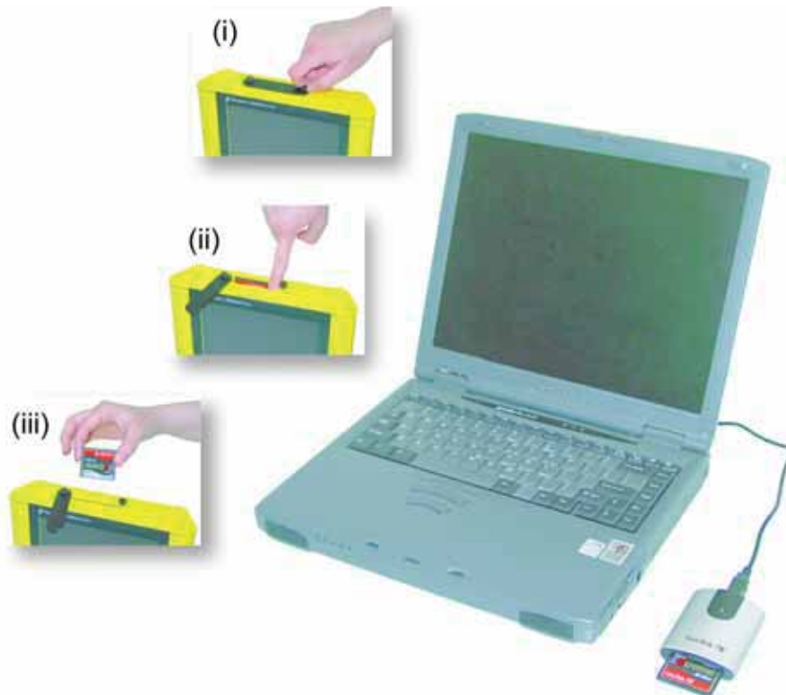
Figure: 13-15 Noggin data files saved to the removable drive are easily transferred to a PC. First, power down the DVL, then (i) loosen both of the finger-screws on the top of the DVL so the drive door can swing open freely. (ii) Press the button to partially eject the compact flash drive. (iii) Remove the drive and insert it into a PC card reader (user supplied). Copy the Noggin data files from the drive into a folder on the PC using the Windows Explorer program. The EKKO_View program can then be used to view the Noggin data.
