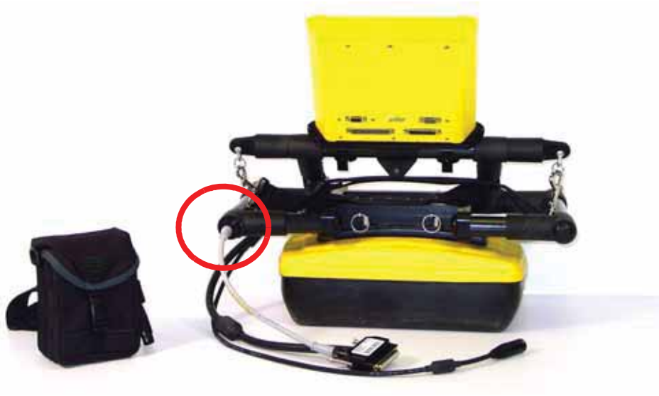
Figure: 8-12 Connect the end of the grey cable to the receptacle on the handle at the back of the frame. This receptacle is adjacent to the Smart button.
