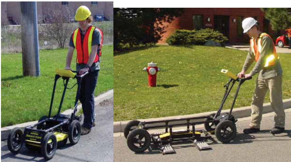
Figure: 5-2 Noggin 250 SmartCart (left) and Noggin 100 SmartCart (right) in operation.
