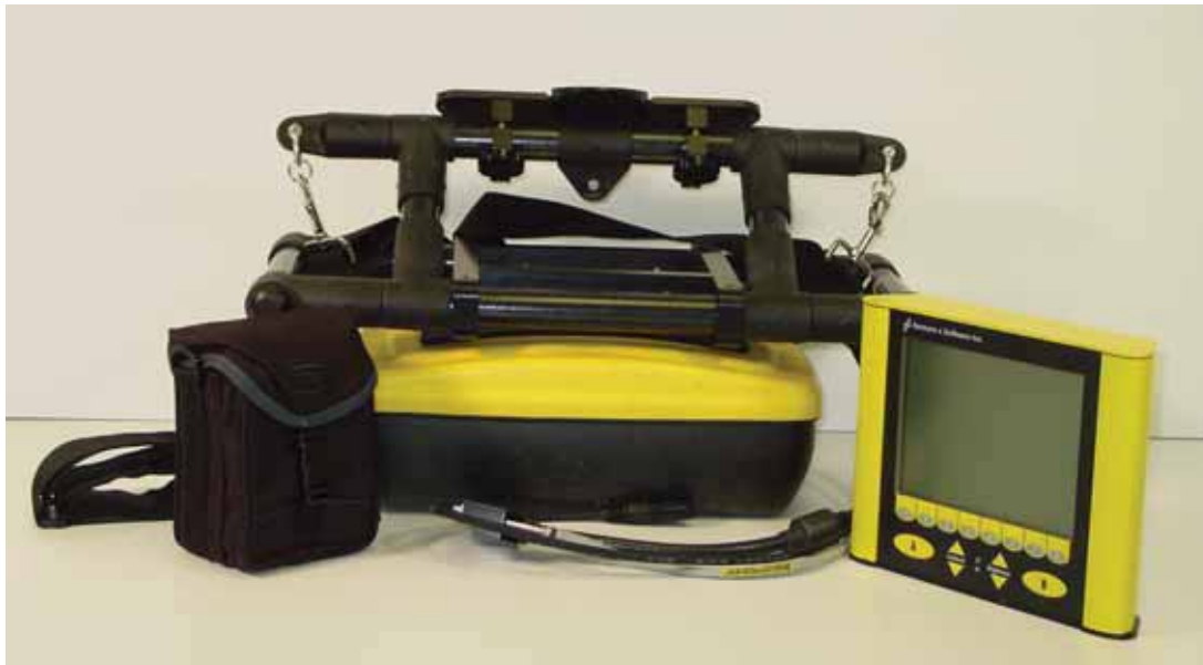
Figure: 8-3 The Rock Noggin system components after removal from the shipping case. From left to right are the belt battery, the Noggin already attached to the frame and the Digital Video Logger (DVL). The system comes partially assembled. To continue with assembly from this point, see Figure 8-11 and later.
