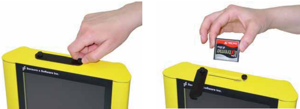
Figure: 10-1 The DVL has a removable compact flash drive for data storage.
