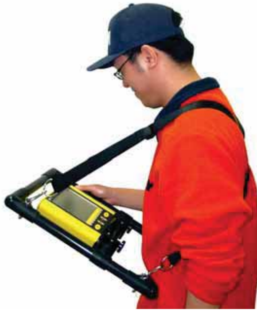
Figure: 10-2 The DVL and control module can be attached to the optional DVL Carrier for hands-free operation. The DVL can be adjusted to optimize the view angle.
