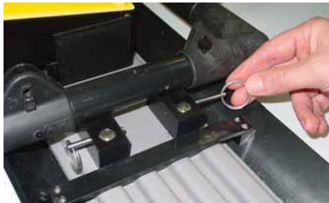
Figure: 6-6 Secure the SmartTow frame to the Noggin 100 by inserting the metal pins into each of the 8 post blocks.
