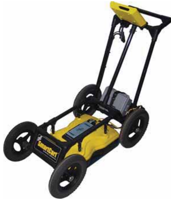
Figure: 5-1 Fully assembled SmartCart with a Noggin 250.
