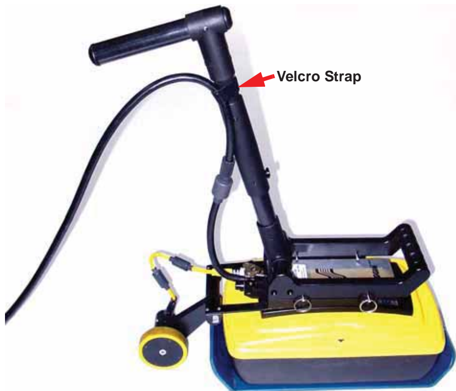
Figure: 7-6 The full-length SmartHandle is shown in Figure 7-1. The SmartHandle can be shortened by removing the center handle section using the thumb-screws. Use the Velcro straps to secure the cable onto the SmartHandle, ensuring there is excess cable near the connection at the Noggin to allow the SmartHandle to pivot up and down without straining the cable.
