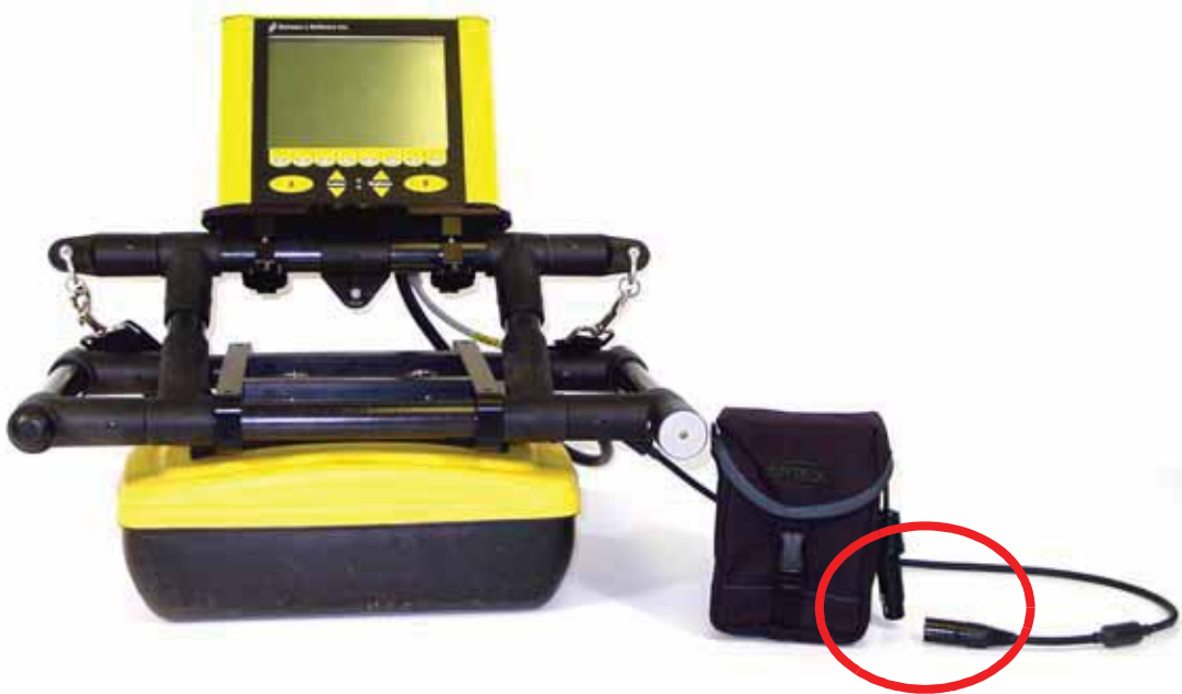
Figure: 8-14 The last connection on the cable is a cylindrical, 4 pin connector for the battery.
