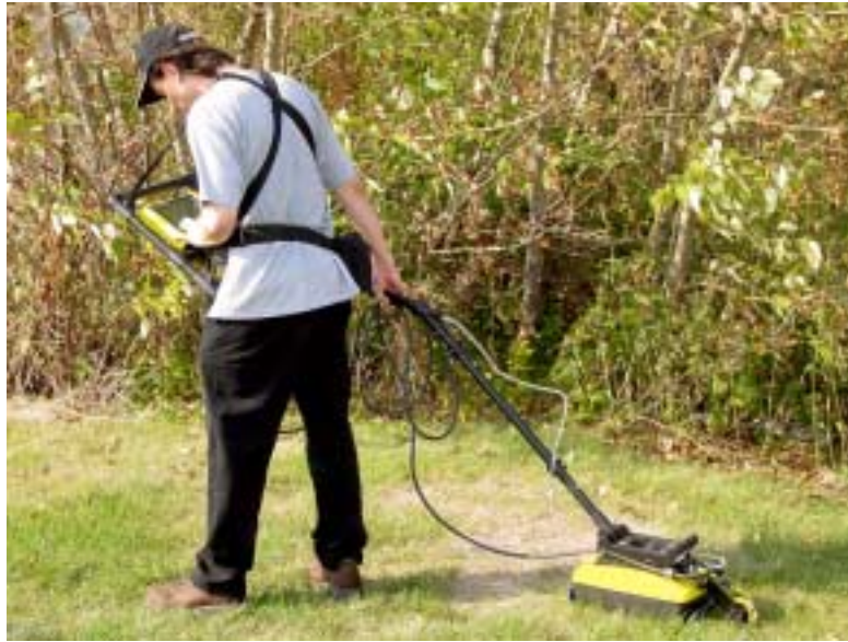
Figure: 6-7 In conditions where pushing the SmartHandle is difficult, it is possible to turn the handle around and pull the system as shown.
