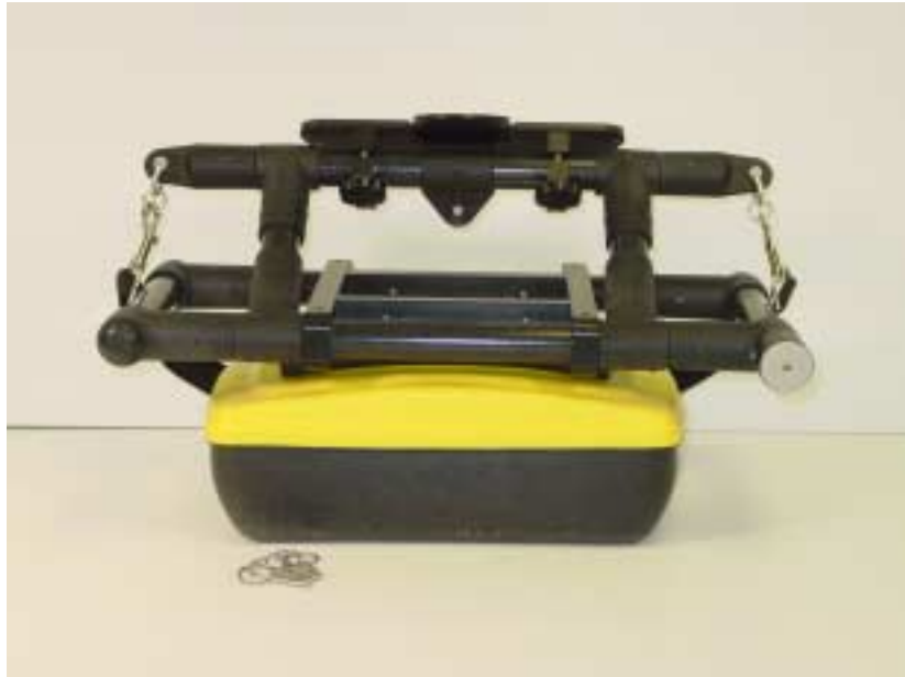
Figure: 7-8 Using the 4 holes on the bottom of the Rock Noggin frame, place the frame on the 4 mounting posts on the top of the Noggin (shown in Figure 7-6). Push the frame down until it cannot go any further. The Noggin should be oriented such that the 37 socket receptacle on the Noggin is on the same side as the Smart button on the frame.
