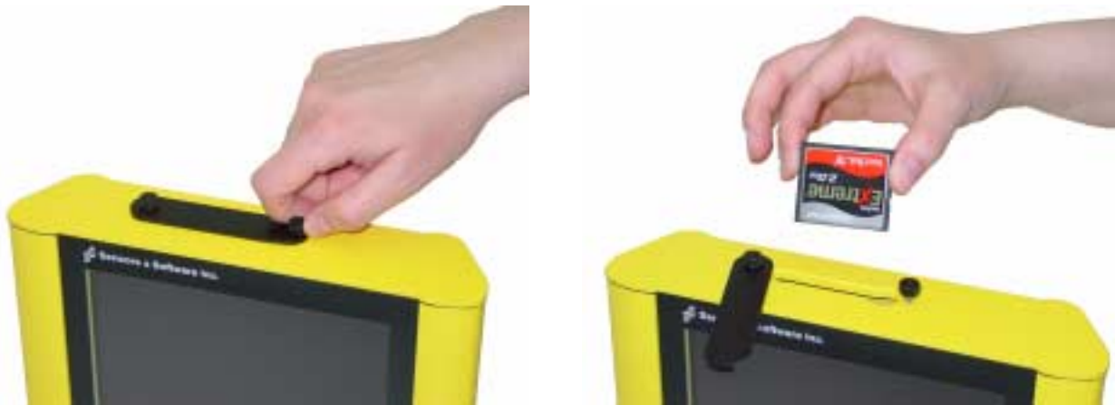
Figure: 9-1 The DVL has a removable compact flash drive for data storage.
