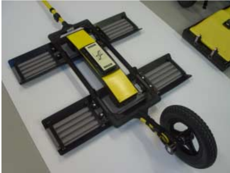
Figure: 5-5 Place the SmartTow frame over the Noggin 100 system with the 8 antenna mounting posts inserted in the post blocks.
