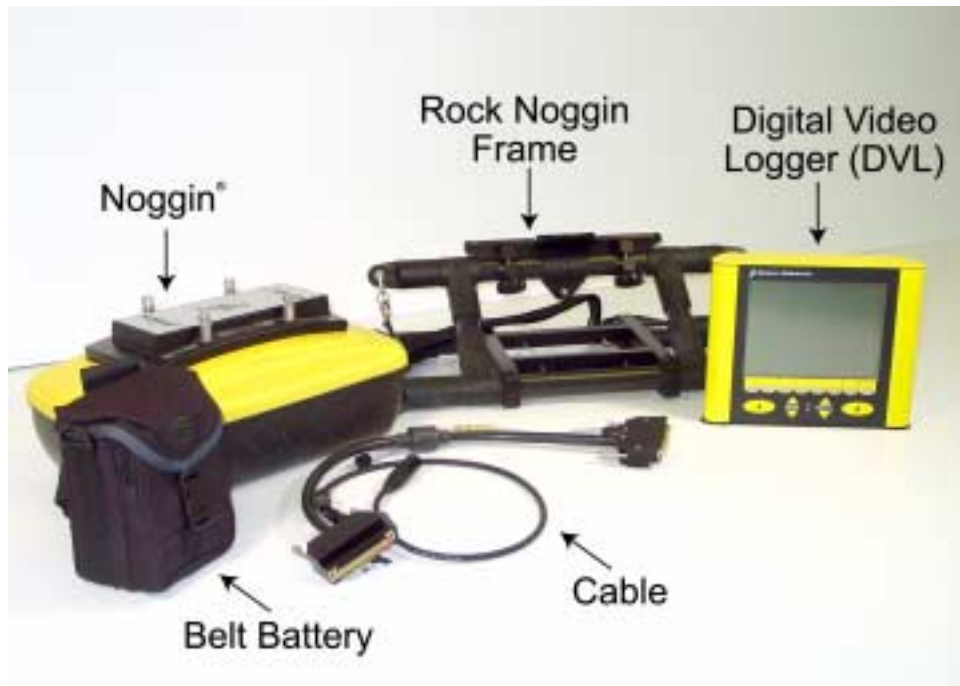
Figure: 7-4 The Rock Noggin system disassembled into its basic components and ready for assembly. From left to right are the belt battery, the Noggin, the cable (in front), the frame and the Digital Video Logger (DVL). More details of each component are given in the figures below.
