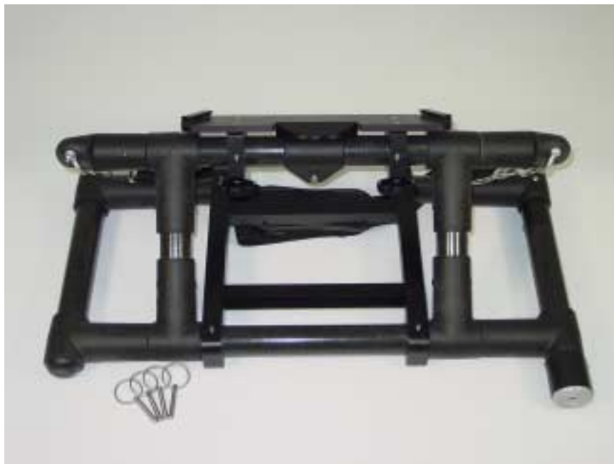
Figure: 7-7 The Rock Noggin frame. On the bottom of the right handle, note the grey speaker that is used to sound an audible tone as data are collected. Also, on the underside of the right handle, note that Smart button (not visible in this view) used to collect data. The frame is attached to the Noggin using the 4 clevis pins shown (see below). The Digital Video Logger (DVL) clips onto the shelf at the top of the frame (see Figure 7-11).
