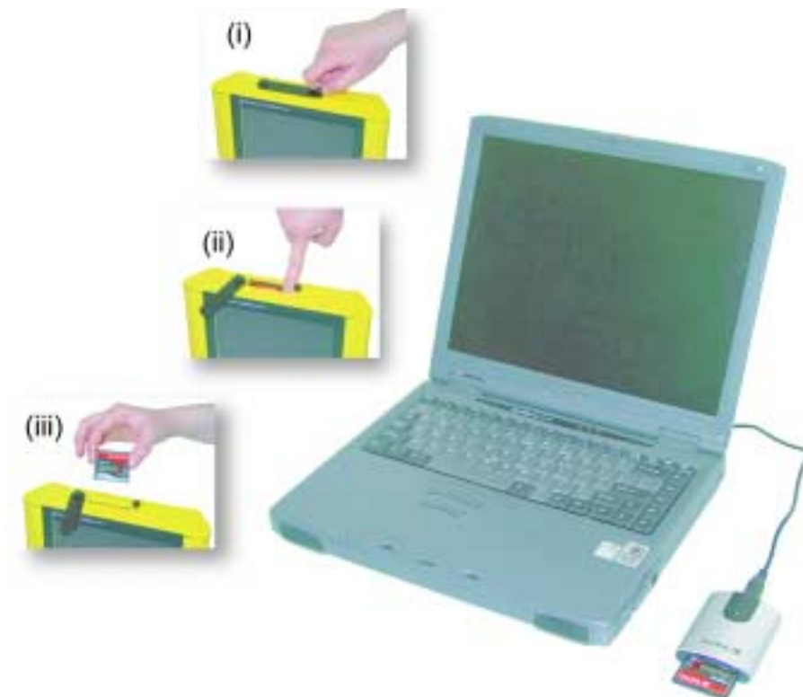
Figure: 12-17 Noggin data files saved to the removable drive are easily transferred to a PC. First, power down the DVL, then (i) loosen both of the finger-screws on the top of the DVL so the drive door can swing open freely. (ii) Press the button to partially eject the compact flash drive. (iii) Remove the drive and insert it into a PC card reader (user supplied). Copy the Noggin data files from the drive into a folder on the PC using the Windows Explorer program. The WinPXFER program can then be used to view the Noggin data.
