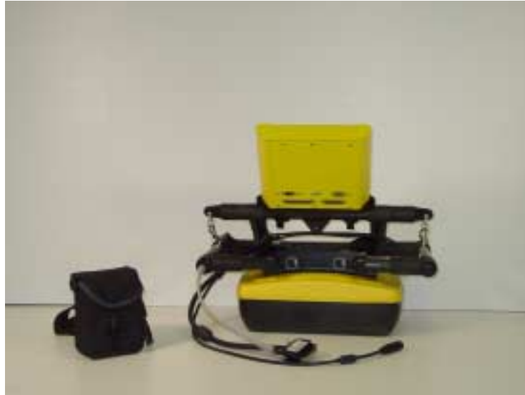
Figure: 7-12 Connect the end of the grey cable to the receptacle on the handle at the back of the frame. This receptacle is adjacent to the Smart button.
