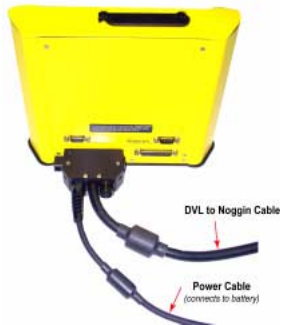
Figure: 9-3 The DVI-to-Noggin cable connects to the back of the DVL.
