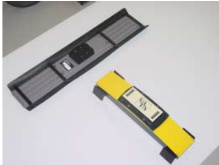
Figure: 3-1 Noggin 100 assembly of electronics to antenna.
