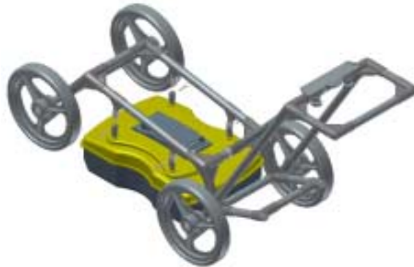
Figure: 4-9 Attaching the Noggin 250 to the SmartCart.
