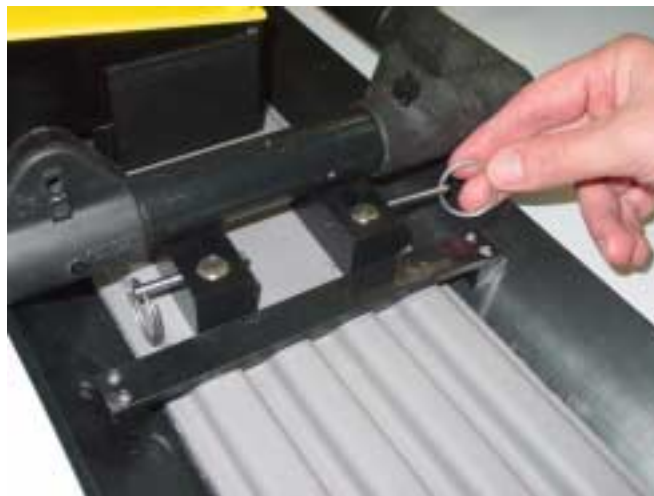
Figure: 5-6 Secure the SmartTow frame to the Noggin 100 by inserting the metal pins into each of the 8 post blocks.
