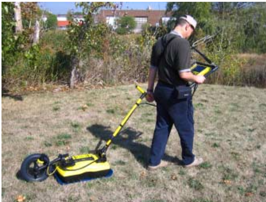
Figure: 5-9 Noggin 250 SmartTow in operation. Note the belt battery used to power the system.
