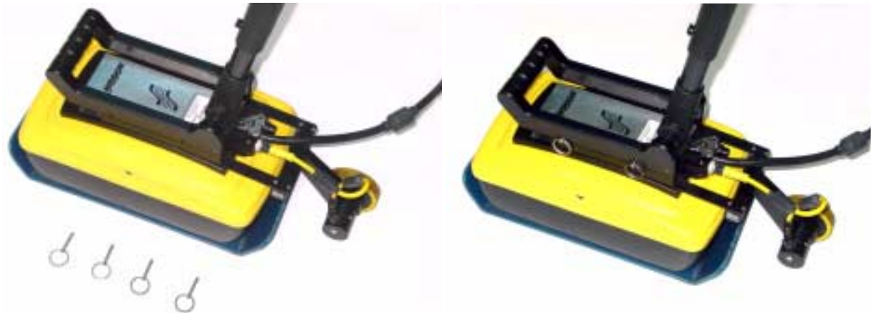
Figure: 6-5 Press the handle base straight down onto the four, silver mounting posts. The handle base should be pushed all the way down onto the odometer bracket. Insert the four quick release pins to secure the handle.
