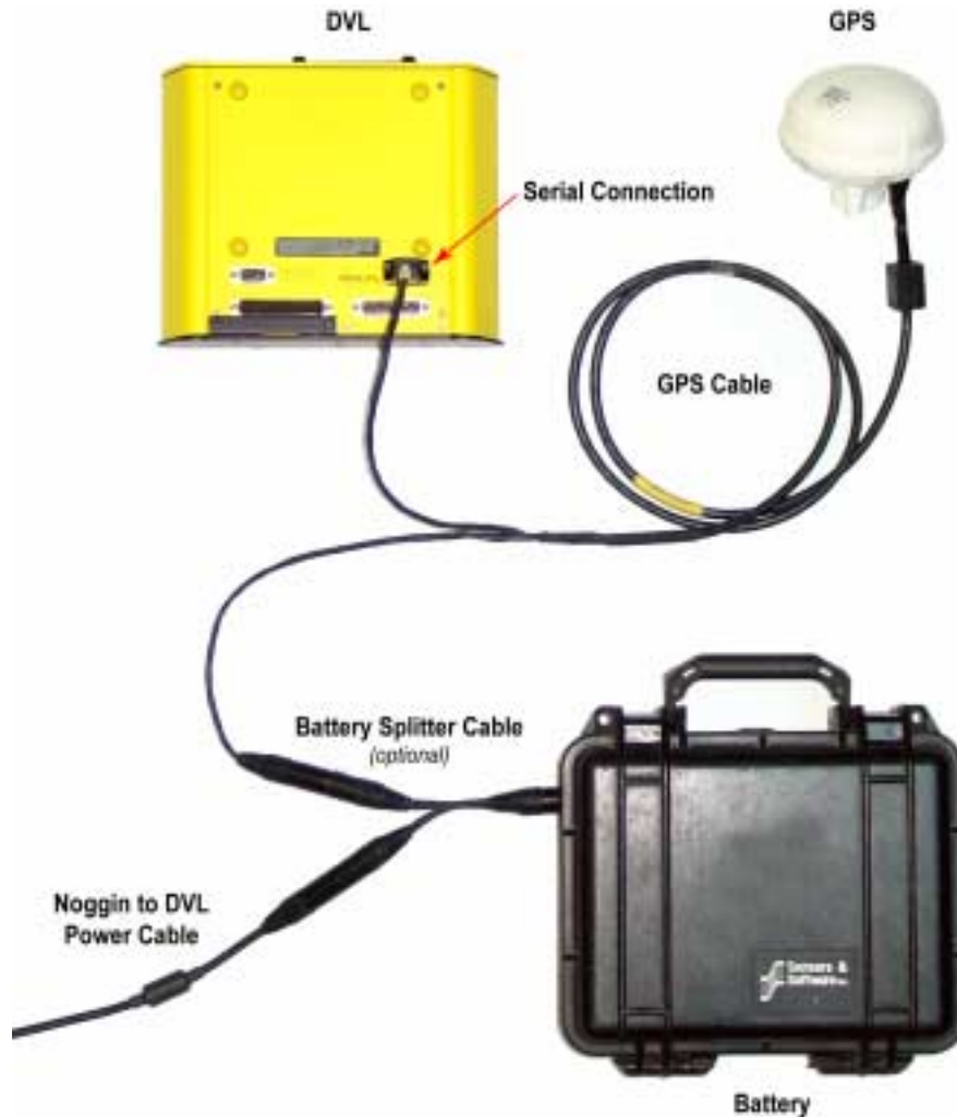
Figure: 8-1 GPS connect to the back of the DVL using a serial connection. GPS supplied with IceMap come with a battery splitter cable to power the GPS from the IceMap battery.
