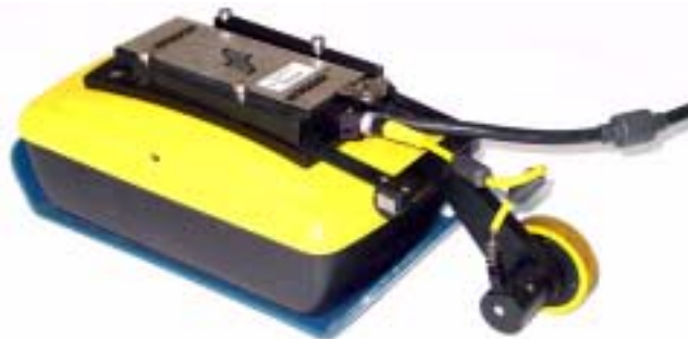
Figure: 6-4 On the Noggin-to-DVL cable, note the round receptacle on the back of the connector that attaches to the Noggin unit. Connect the yellow odometer cable to this round receptacle.
