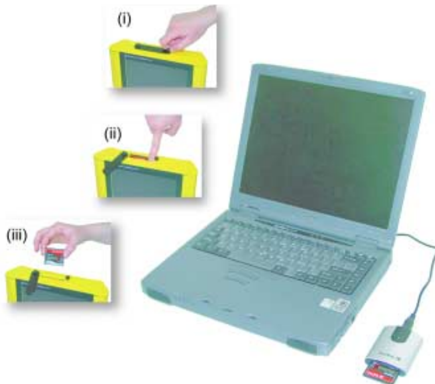
Figure: 12-17 Noggin data files saved to the removable drive are easily transferred to a PC. First, power down the DVL, then (i) loosen both of the finger-screws on the top of the DVL so the drive door can swing open freely. (ii) Press the button to partially eject the compact flash drive. (iii) Remove the drive and insert it into a PC card reader (user supplied). Copy the Noggin data files from the drive into a folder on the PC using the Windows Explorer program. The WinPXFER program can then be used to view the Noggin data.
