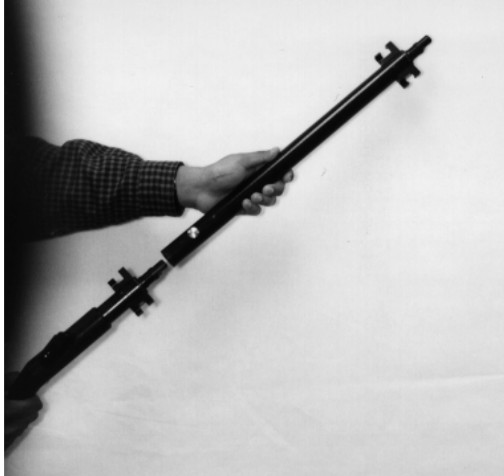
Figure 3-2: Simply push the Smart Handle grip into the Smart Handle extension
