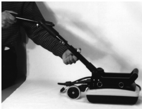
Figure 3-6: To separate either the short or long handle from the Noggin, press on the large grey
