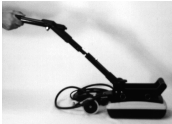
Figure 3-5: If short handle is required, it may be easier to just connect the SmartHandle grip to the Noggin without the extension.
