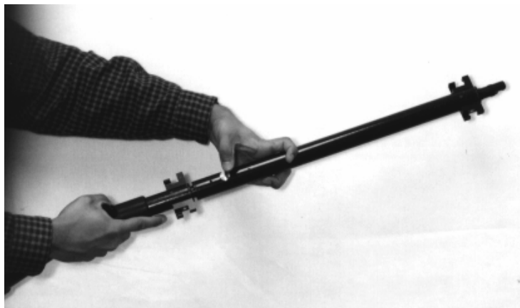
Figure 3-3: To separate them, push on the large grey button on the extension and pull them apart
