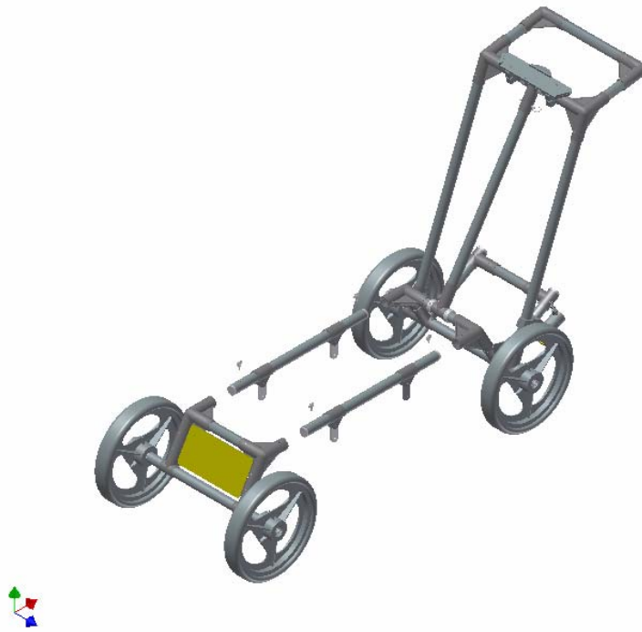
Figure 2-13: Changing the Smart Cart's support arms to carry a different Noggin system.
