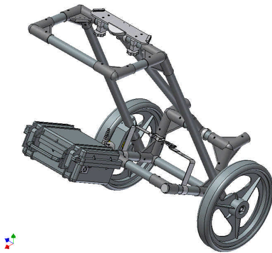
Figure 2-9: The Noggin Smart Cart battery.
