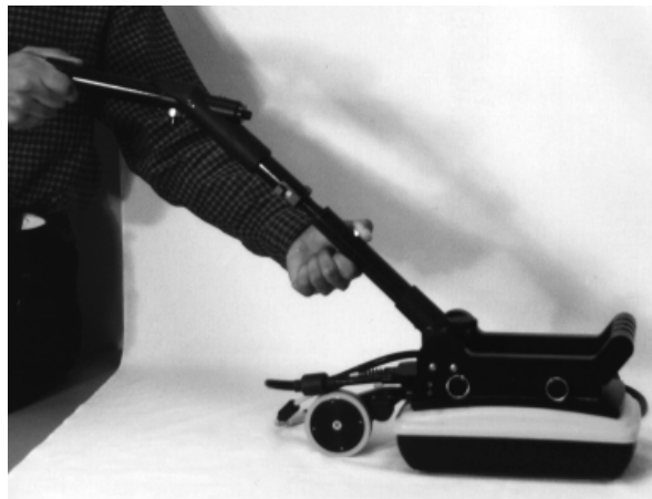
Figure 3-6: To separate either the short or long handle from the Noggin, press on the large grey button on the pole extending from the Noggin and pull apart.
