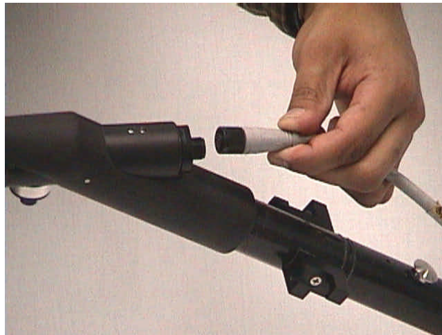
Figure 3-8: The Smart Grip Cable attaches to the end of the Smart Handle Grip. This connects the Smart Handle button (extreme left, bottom) and beeper (not shown) into the system.
