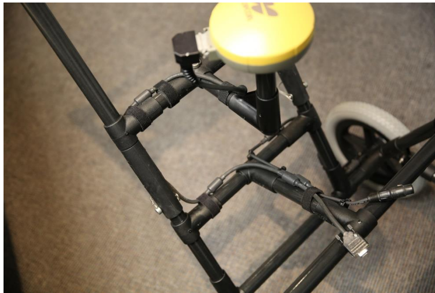
Figure 2-12: Make sure the GPS cable is routed as shown and secured to the cart, as it moves from the PDP sensor up to the GPS receiver along the cart frame.
