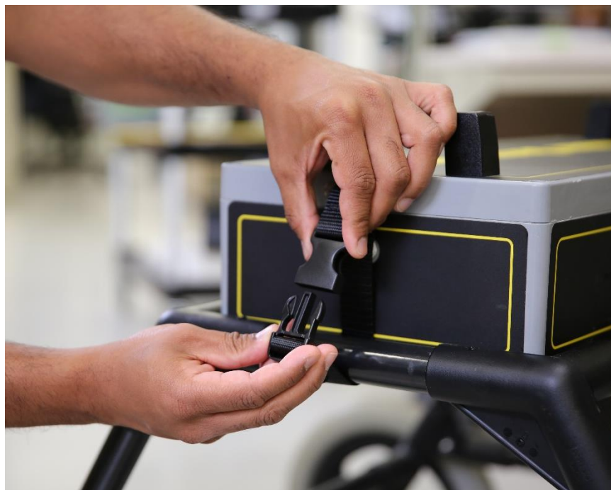
Figure 2-5: Secure PDP sensor with straps on either end
