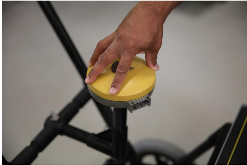
Figure 2-10: Screw the Topcon GPS receiver onto the GPS mount
