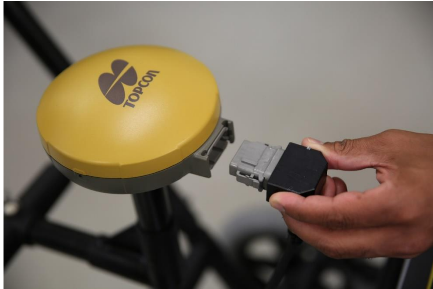
Figure 2-13: Plug the GPS cable into the GPS receiver
