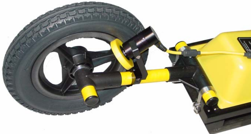
Figure 2-23: The big wheel odometer attaches to the skid plate assembly exactly the same way as the adjustable tow handle is attached. Place the T end of the odometer into the trough on the end of the skid plate assembly. The labels on the transmitting transducer should be facing away from this end. The T end of the odometer is attached to the skid plate assembly by placing the U-bracket over the top and into the vertical slots. The odometer is secured into place by inserting the metal pins into the holes at the bottom of the U bracket.
