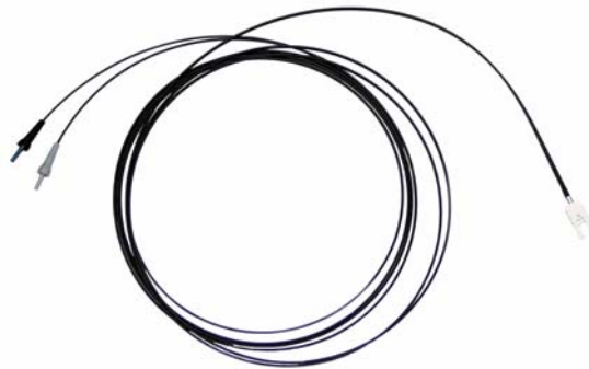
Figure 2-16: Dual fibre optic cable used with the transmitter and receiver. The black and grey strain reliefs on the end of the cable (left) plug into the same coloured fibre optic receptacles on the top of the transmitter and receiver (see Figure 2-17). The connection on the other end of the cable (right) connects to either fibre optic receptacle on the control module (see Figure 2-18).
