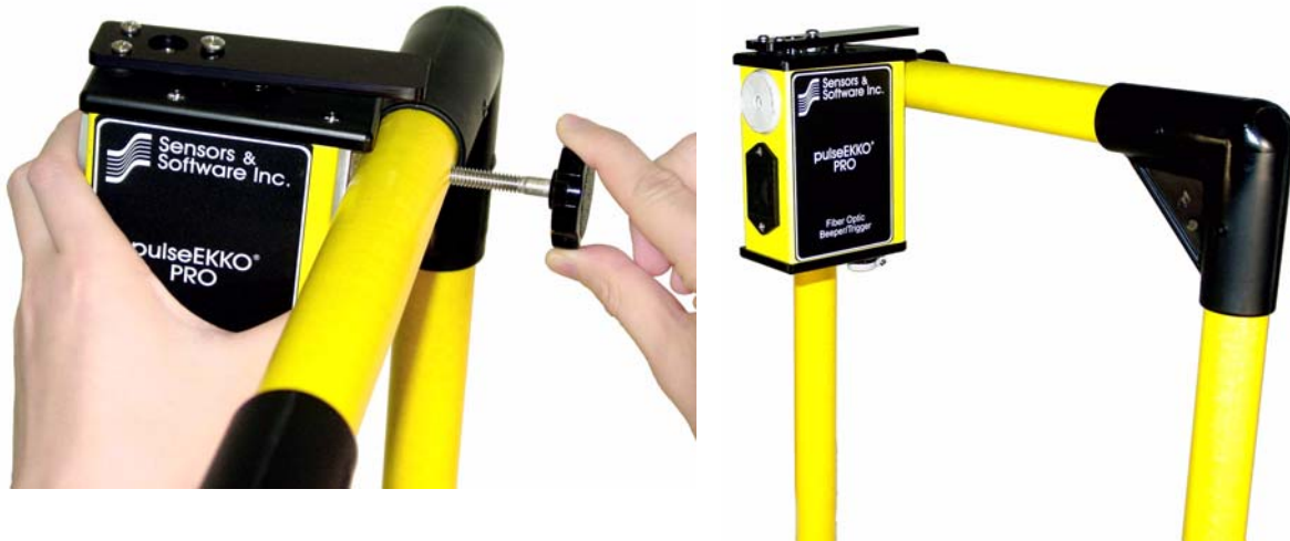
Figure 2-28: Attaching the Fibre Optic Remote Beeper/Trigger unit to the transmitter handle.
