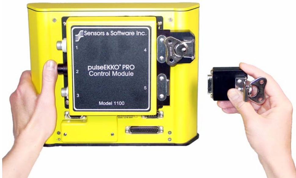
Figure 2-6: Low frequency antennas (12.5 to 200 MHz) require the electrical to fibre optic converters to be attached to the control module and secured using the latches.
