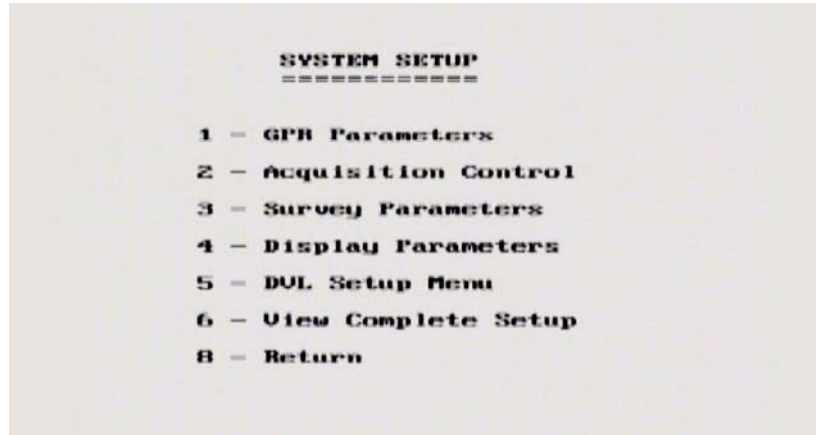
Figure 3-1: The System Setup main menu is used to access and change any parameter used for data collection. Related parameters are grouped under different menu headings, for example, GPR Parameters list the variables specific to the GPR system. Select View Complete Setup from this menu to quickly locate the desired parameter and the heading it is listed under.
