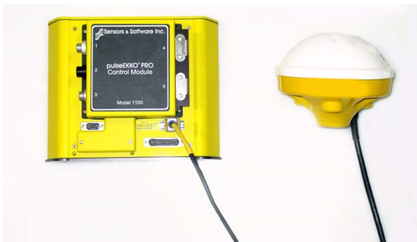
Figure 2-33: Attaching a GPS to the serial port on the back of the DVL.
