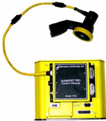
Figure 2-32: The pulseEKKO PRO accepts input from various odometers including the wheel odometer shown in the figure, which is typically used with the SmartCart. Odometers attach to receptacle 1 on the control module.
