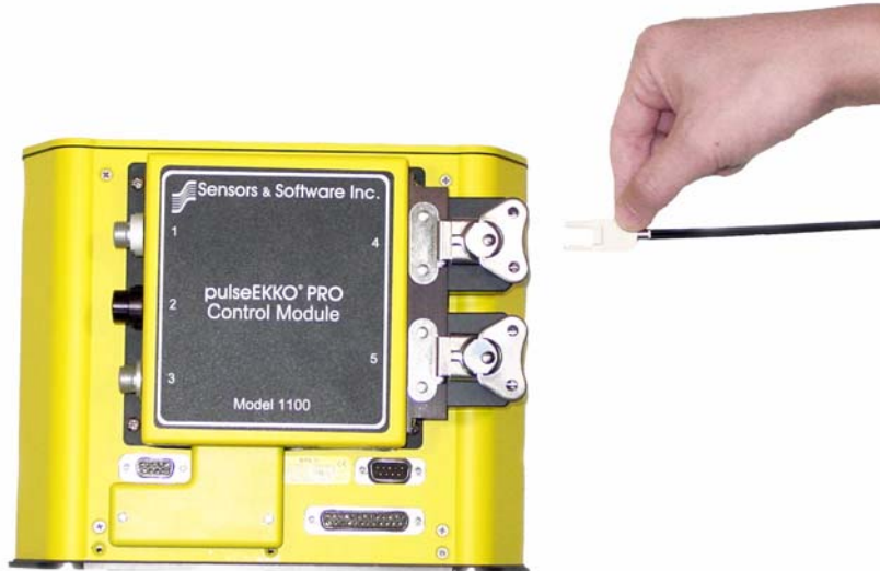
Figure 2-18: The dual fibre optic cable from the transmitter and receiver attaches to the electrical to fibre optic converters on the control module. The fibre optic cable from the transmitter connects to the control module receptacle labelled 4 while the fibre optic cable from the receiver connects to the control module receptacle labelled 5. This connection is keyed so it will only attach when the fibre optic cable is in the orientation shown.
