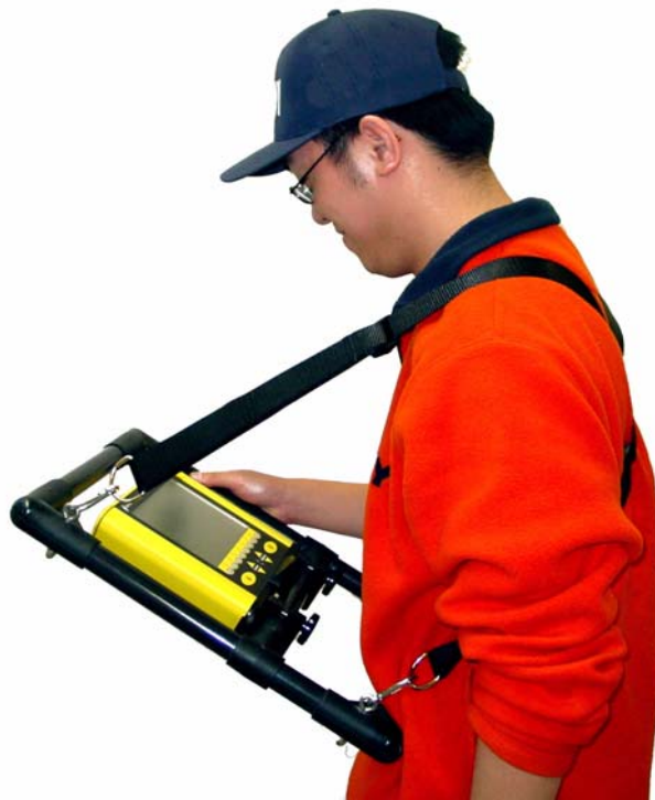
Figure 2-31: The DVL and control module can be attached to the optional DVL Carrier for hands-free operation. The DVL can be adjusted to optimize the view angle.
