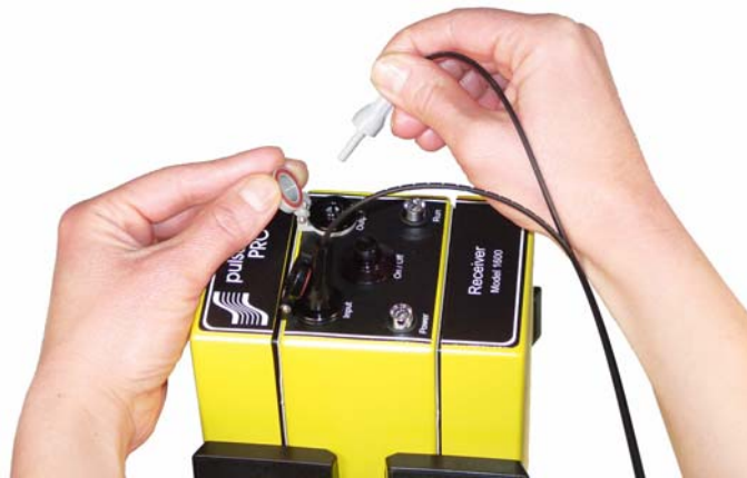
Figure 2-17: Attaching the fibre optic cables to the transmitter and receiver. Make sure to match the connector colour to the door colour (grey to grey and black to black). Push the fibre optic cable down until you can feel it “click” into place.
