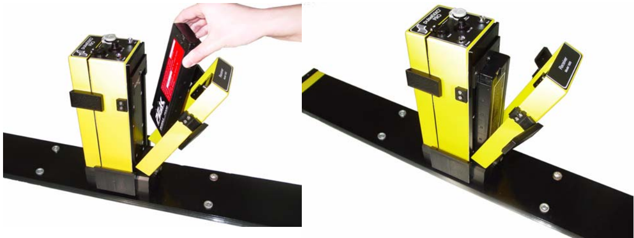
Figure 2-13: Insert the 12 Volt battery into the battery compartment making sure that battery polarity is correct. The positive (+) terminal faces inward. The battery is “keyed” so it will only seat properly in the compartment if it is in the correct orientation.
