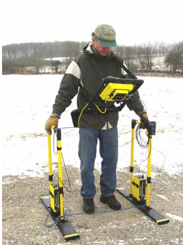
Figure 6-2: One person operation setup. The operator moves the antennas to each data location point and collects the trace using the fibre optic beeper trigger. The data are visible in real time on the DVL screen.
