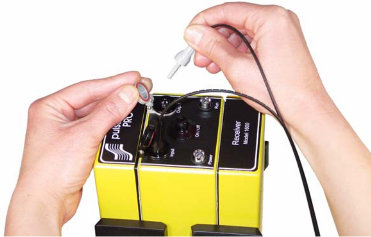
Figure 7-2: Make sure fibre optic strain relief colour matches the receptacle door colour (grey to grey and black to black).
