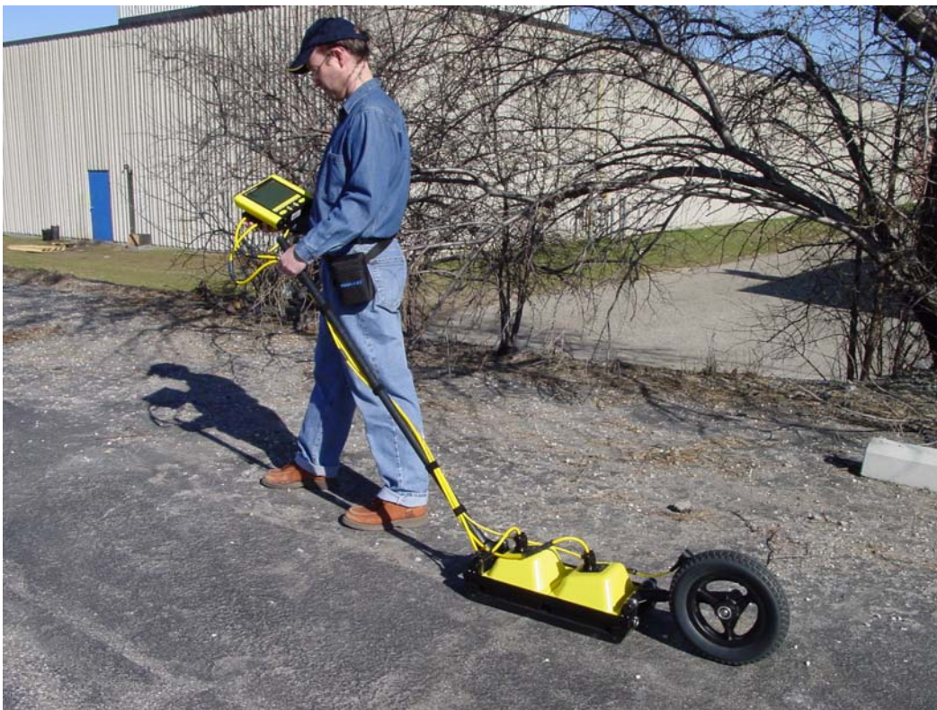
Figure 6-5: High frequency tow mode operation. As the operator drags the transducers across the surface, the odometer triggers data collection at equally-spaced intervals (called the Step Size). The data being collected are visible in real time on the DVL screen.
