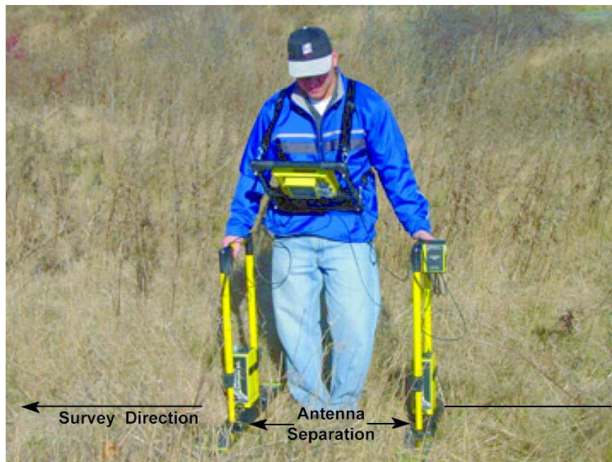
Figure 6-7: Most common reflection surveying technique. Antennas are held at the proper antenna separation for the selected frequency and perpendicular to the survey line direction. This antenna orientation ensures the maximum in-line GPR energy and reduces reflections from off-line targets.
