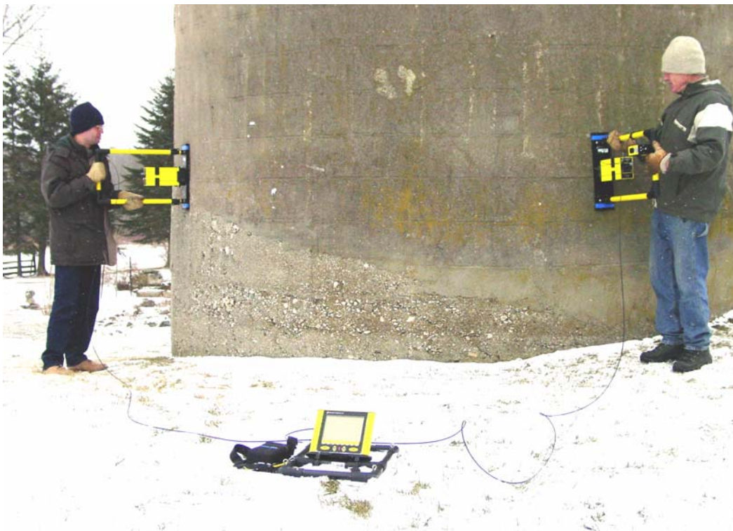
Figure 6-14: Transillumination survey setup. With a transillumination survey, the GPR signal is sent from the transmitter directly to the receiver after it has passed through a structure. The DVL is centrally located and data acquisition is controlled by either triggering the system with the electrical or fibre optic beeper/trigger or using Free Run mode with a time delay between traces.
