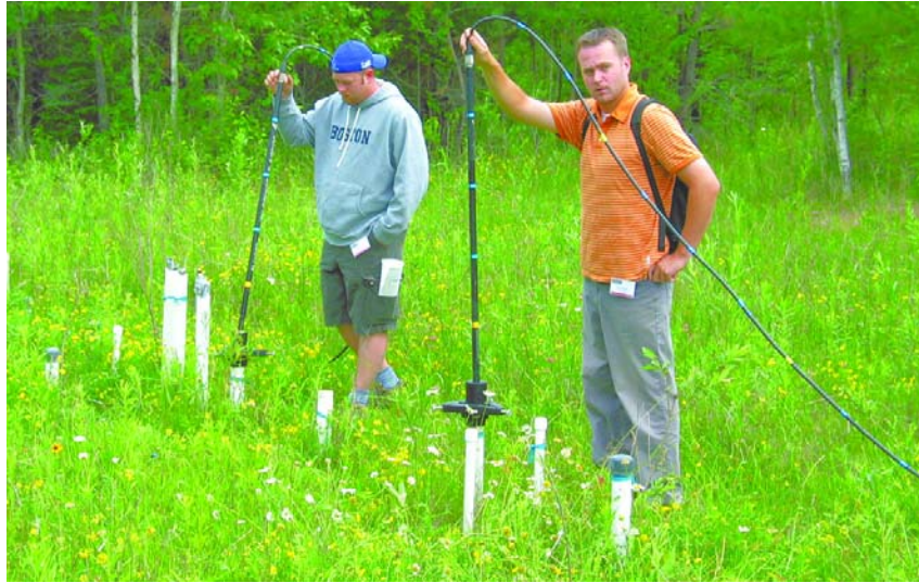
Figure 6-13: Cross hole transillumination surveys with the pulseEKKO PRO system require the use of 50, 100 or 200 MHz bore-hole antennas available from Sensors & Software.
