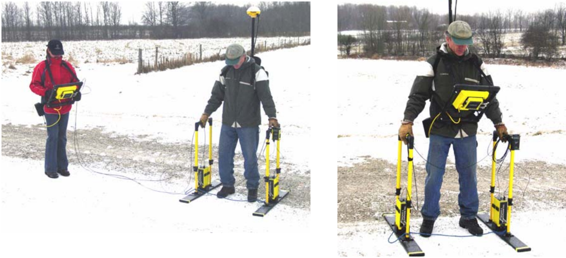
Figure 6-9: Two person (left) and one person (right) system configurations with GPS added. Ideally, the GPS should be positioned near the mid-point of the GPR antennas.
