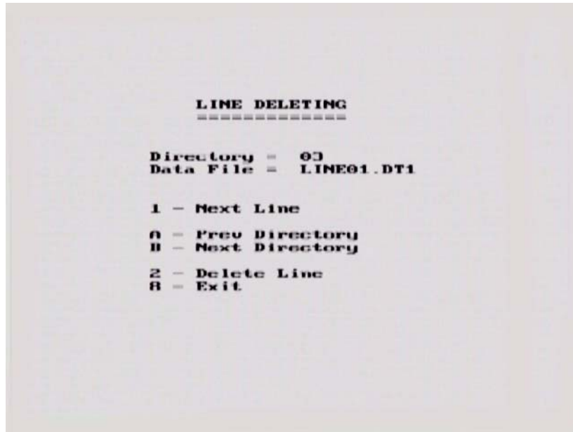
Figure 8-6: Line Delete screen. Use the A and B button to select one of the 20 available directories, then use the 1 button (Next Line) to move through the data lines in the directory. When the name of the data line to transfer appears, press 2 (Delete Line) to delete the line from the directory.
