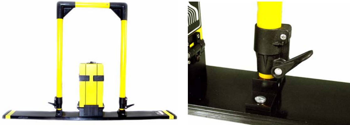
Figure 2-14: Attach the adjustable handles to the antennas by tightening the 4 quarter-turn fasteners. Adjust the height of the handle by loosening the levers at the base of the handles (right) and pulling the handles up to the correct height.
