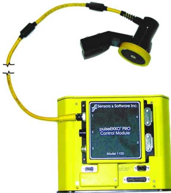
Figure 2-24: The Big Wheel Odometer uses a long extension cable (not shown) to attach to receptacle 1 on the control module.
