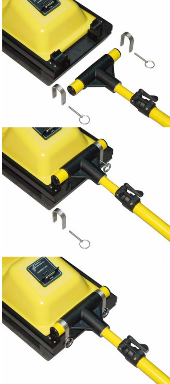
Figure 2-21: To attach the adjustable tow handle to the skid plate assembly, place the T end of the handle into the trough on the end of the skid plate assembly where the receiving transducer label is facing. The T end of the handle is attached to the skid plate assembly by placing the U-bracket over the top and into the vertical slots. The handle is secured into place by inserting the metal pins into the holes at the bottom of the U bracket.
