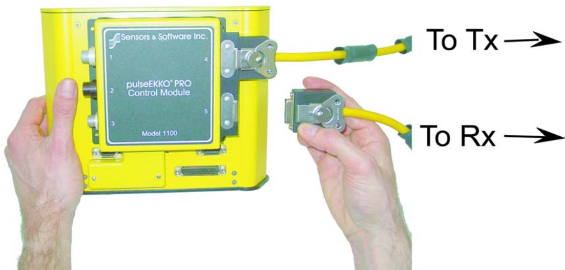
Figure 2-26: Connecting the transducer cables to the Control Module. The transducer cable from the transmitting transducer connects to the control module receptacle labelled 4 while the transducer cable from the receiving transducer connects to the control module receptacle labelled 5. The cable attachments are secured with latches.
