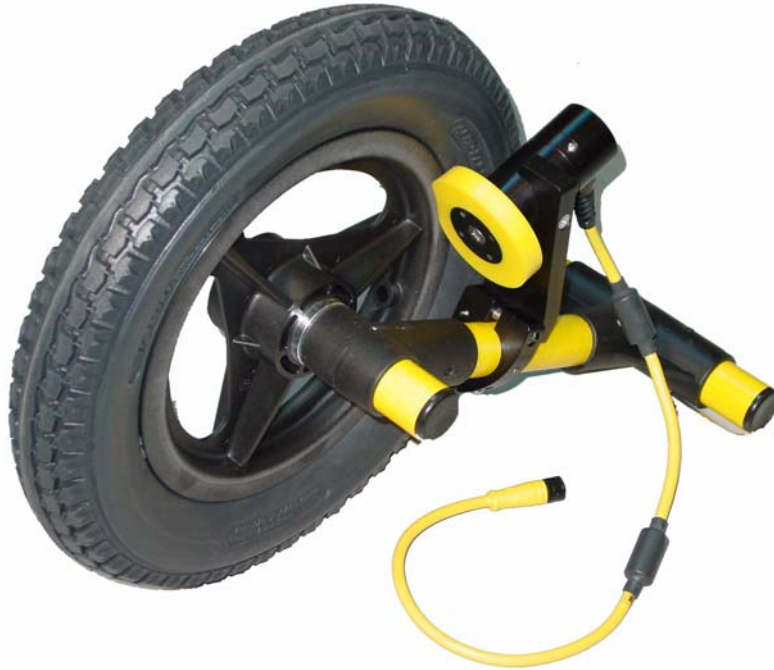
Figure 2-22: The big wheel odometer. Ensure that the small yellow odometer is tightly pressed against the rim of the wheel so that it spins when the big wheel is rotated.
