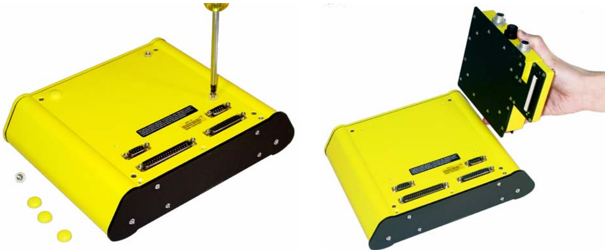
Figure 2-4: Remove the 4 yellow caps and the 4 screws from the back of the DVL (left) and place the control module on the back of the DVL (right). Make sure that the 37 pin connector is aligned properly with the 37 socket connector on the control module.
