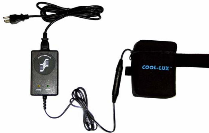
Figure 7-3: Belt battery (right) used to power the DVL and Control Module. The battery charger is shown on the left.
