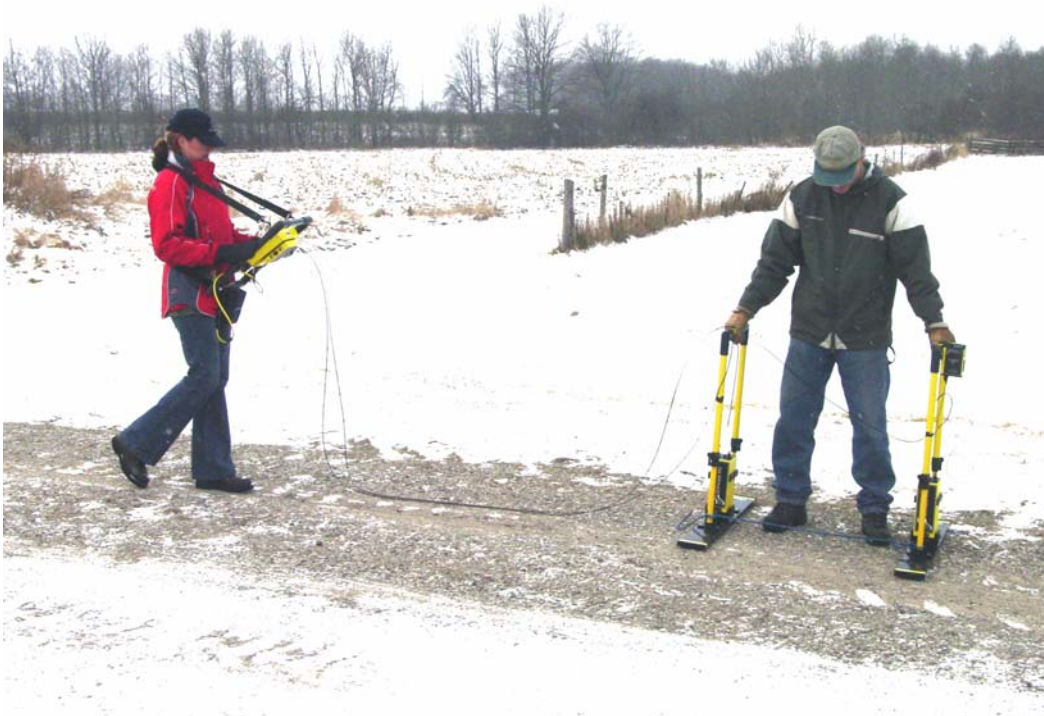
Figure 6-1: Two person data collection with the pulseEKKO PRO system. The antenna operator moves the antennas to each data location point. The data trace is collected by the DVL operator using the electrical beeper/trigger or the DVL button. The data trace can also be collected by the antenna operator using the fibre optic beeper/trigger. The data are visible in real time on the DVL screen.
