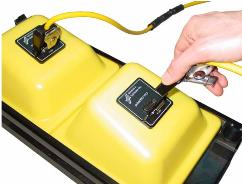
Figure 2-25: Connecting the transducer cables to the transducers. The connections are secured with latches.
