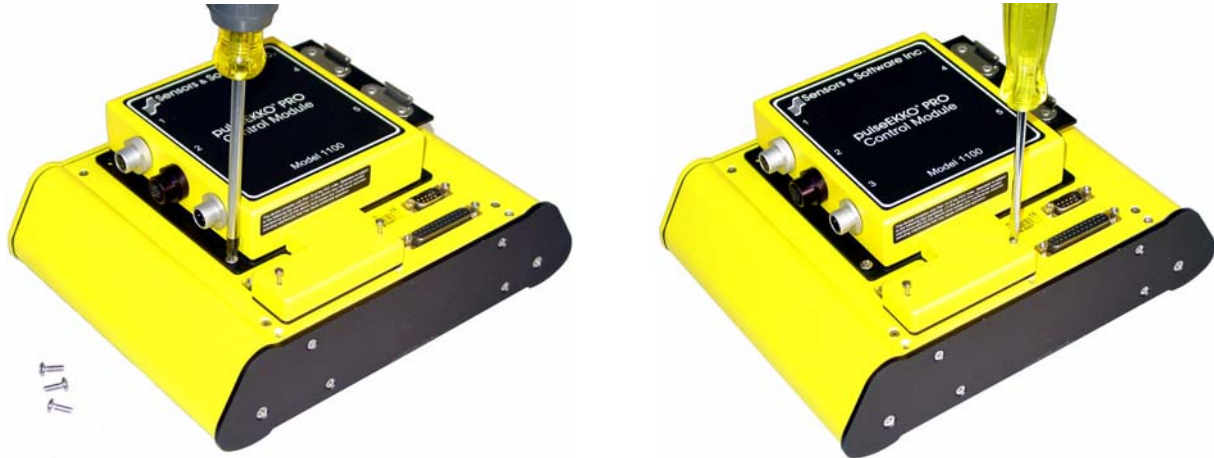
Figure 2-5: Attach the control module to the DVL using the 4 screws supplied (left) and a Phillips screwdriver (not supplied). Tighten the 37 pin connectors into place (right) with a small slotted screwdriver (not supplied).
