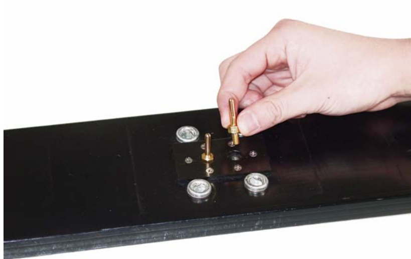
Figure 2-9: Insert the male brass antenna pins into the holes on the top of the antenna and finger-tighten.
